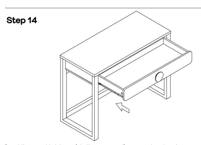
Insert the assembled drawer into the corresponding compartment as shown. Ensure the drawers slide easily along the rails.
