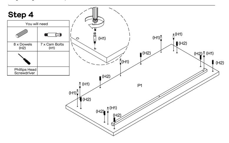
Insert 8 x Dowels (H2) into the Top Panel (P1).
