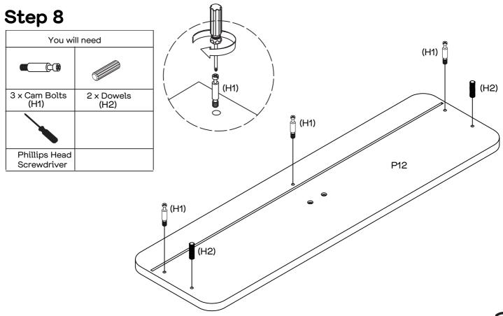
Insert 3  $\times$  Cam Bolts (H1) into the Drawer Front Panel (P12), by tightening with a Phillips Head Screwdriver. Insert 2  $\times$  Dowels (H2) into the Drawer Front Panel (P12).
