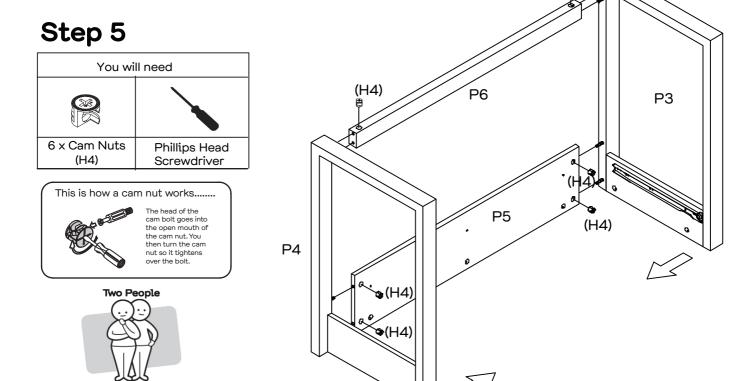
Insert 6 x Cam Nuts (H4) into the Back Panel (P5) and Support Panel (P6). Rotate the Cam Nuts so the arrows point towards the incoming cam bolts. Attach the Base Panel (P5) and Support Panel (P6) to the Left Side Panel (P3) and Right Side Panel (P4), by tightening all Cam Nuts with the Phillips Head Screwdriver.
