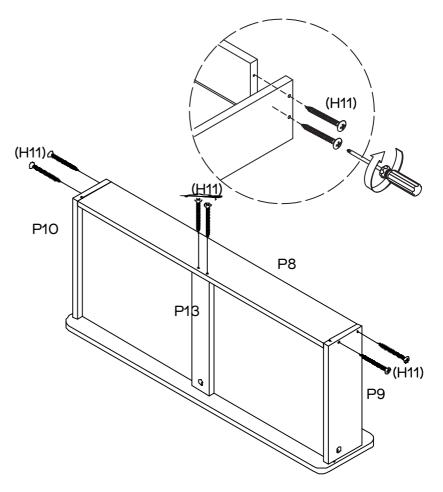
Attach the Drawer Back Panel (P8) to the Drawer Side Panels (P9 & P10) and Drawer Support Panel (P13) with 6 x Drawer Screws (H11), by tightening with a Phillips Head Screwdriver.
