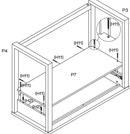
Insert 4 x Dowels (H2) into panels (P3 & P4). Attach the Base Panel (P7) to the panels (P3, P4 & P5) with 7 x Drawer Screws (H11), by tightening with the Phillips Head Screwdriver.
