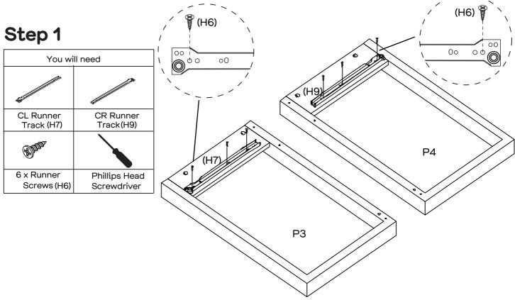
Attach CL Runner Track (H7) to the Left Side Panel (P3) with 3  $\times$  Runner Screws (H6), by tightening with a Phillips Head Screwdriver.
