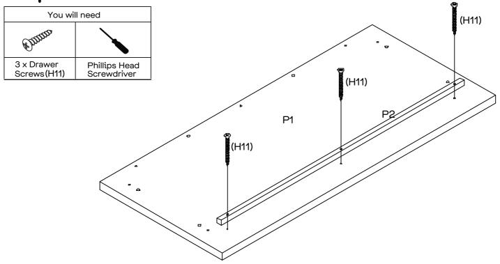
Add the Steel Bar (P2) to the underside of the Top Panel (P1) with  $3 \times 1$  Drawer Screws (H11), by tightening with the Phillips Head Screwdriver.
