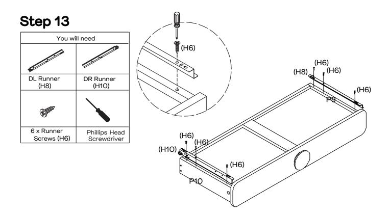
Attach 1 x DL Runner (H8) to the bottom of Drawer Side Panel L (P9) and 1 x DR Runner (H10) to the bottom of Drawer Side Panel R (P10) with 6 x Runner Screws (H6) by tightening with the Phillips Head Screwdriver.
