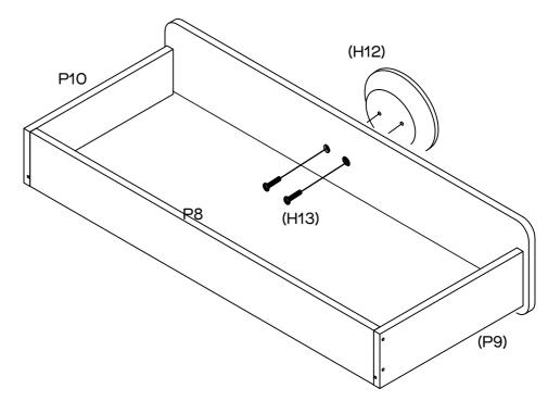
Attach the Handle (H12) to the Drawer Front (P12) with  $2 \times \text{Handle Screws}$  (H13), by tightening with a Phillips Head Screwdriver.
