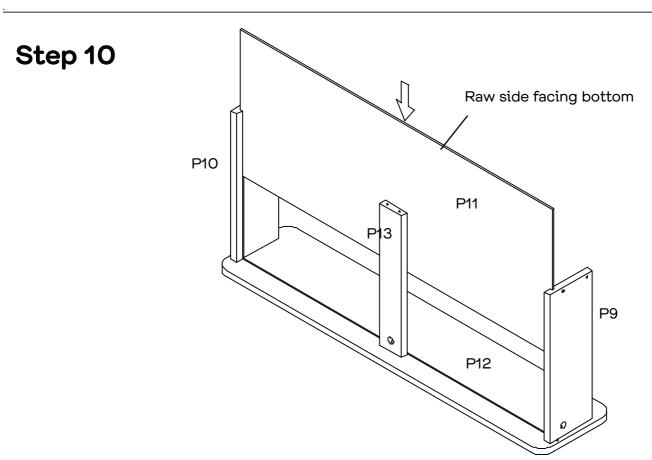
Slot in the Drawer Base Panel (P11) into the grooves of panels (P9, P10 & P11) as shown.
