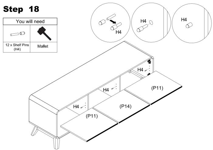
Insert 12 x Shelf Pins (H4) into desired holes in panels. Use a mallet to gently tap them into place if needed. Put Shelf Panels (P11) and (P14) onto shelf pins.
