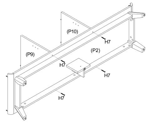
Screw in 4 x Screws (H7) through Bottom Panel (P2) to fasten Panels (P9) & (P10).
