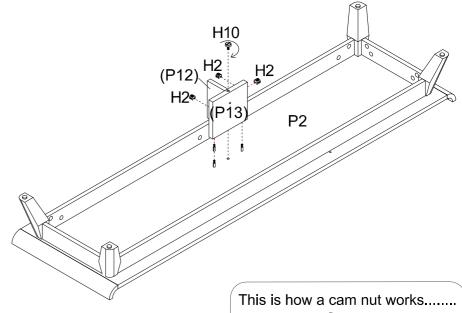
Attach Middle legs (P12) & (P13) to Bottom Panel (P2). Insert 3 x Cam Nuts (H2) into Middle Legs (P12) & (P13). Rotate the cam nuts so the arrows pointing towards the incoming cam bolts and turn clockwise to lock. Screw 1 x Adjustable Foot (H10) to Big Middle Leg (P13).
