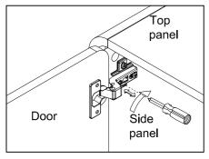
Loosen or tighten the screw indicated a little to adjust the gap between the door panels, adjust the hinge to right position (see step 3a & 3b).
