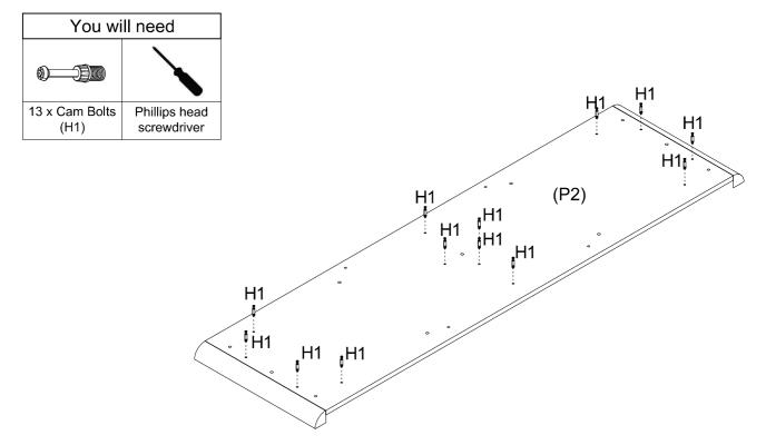
Screw 13 x Cam Bolts (H1) into Bottom Panel (P2) as shown.
