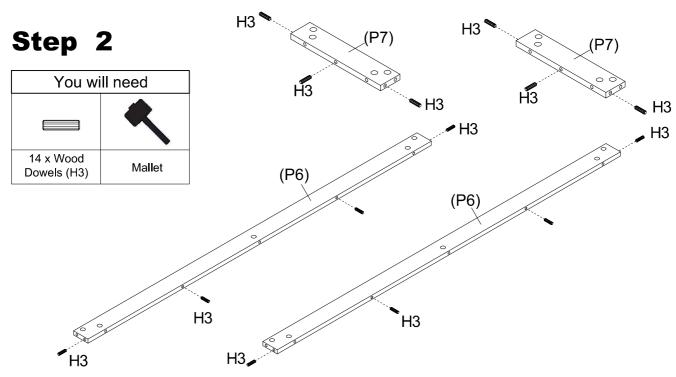
Insert 3 x Wood Dowels (H3) into each Short Rail (P7) and 4 x Wood Dowels (H3) into each Long Rail (P6).
