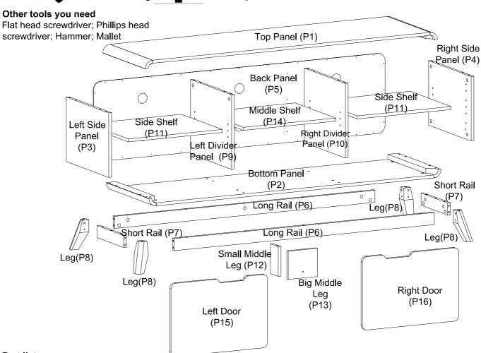
Part list Box 1: Top Panel (P1); Bottom Panel (P2); Back Panel (P5); Long Rail (P6); Short Rail (P7); Leg (P8); Left Divider Panel (P9); Right Divider Panel (P10); Side Shelf (P11); Small Middle Leg (P12); Big Middle Leg (P13); Middle Shelf (P14). Box 2: Left Side Panel (P3); Right Side Panel (P4); Left Door (P15); Right Door (P16).
