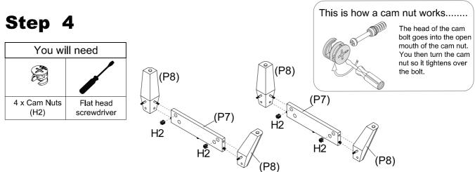
Insert 2 x Cam Nuts (H2) into each Short Rail (P7).
