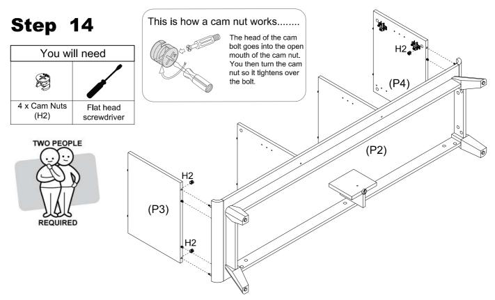
Attach Side Panels (P3) & (P4) to Bottom Panel (P2). Insert 4 x Cam Nuts (H2) into side panels and turn clockwise to lock.
