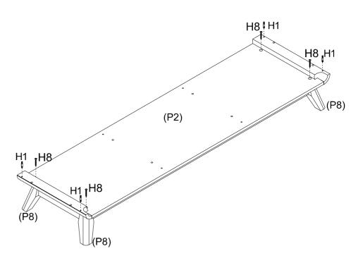
Screw 4 x Cam Bolts (H1) into Bottom Panel (P2) as shown.
