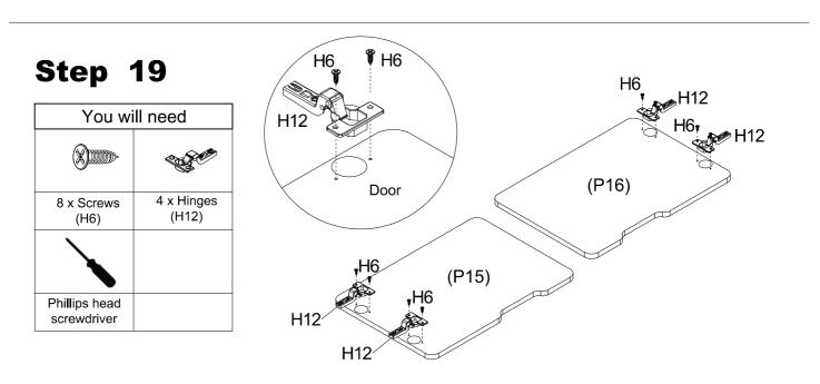
Insert 4 x Hinges (H12) into Doors (P16) and (P15). Attach with 8 x Screws (H6).
