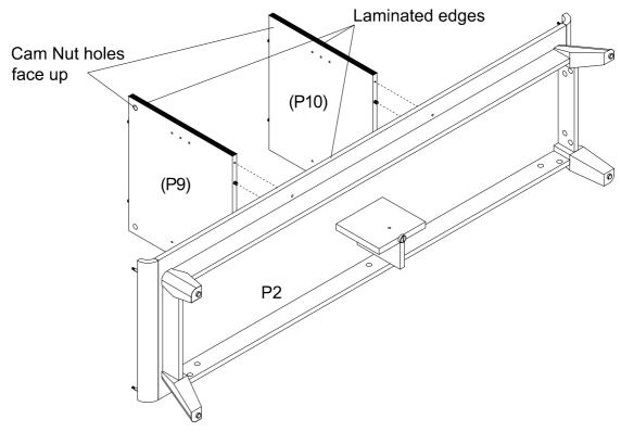
Attach Divider Panels (P9) & (P10) to Bottom Panel (P2).
