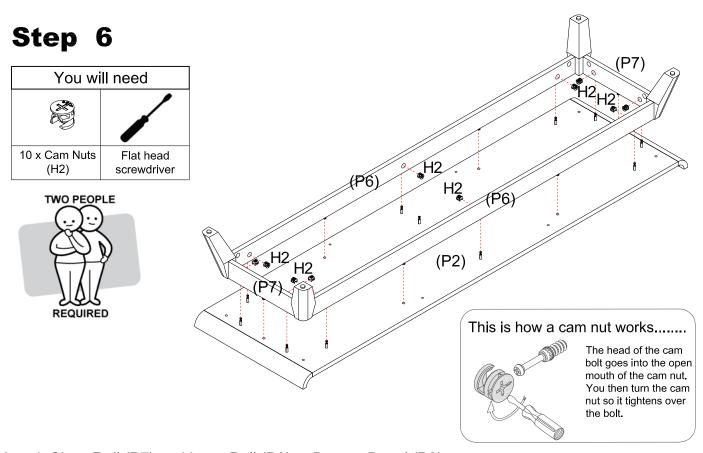
Attach Short Rail (P7) and Long Rail (P6) to Bottom Panel (P2). Insert 10 x Cam Nuts (H2) into Short Rails (P7) and Long Rails (P6) with the arrow pointing towards the incoming bolt, and turn clockwise to lock.
