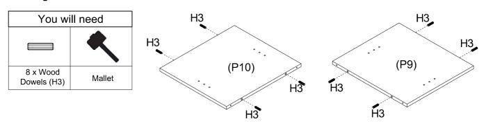
Insert 8 x Wood Dowels (H3) into Left Divider Panel (P9) and Right Divider Panel (P10).
