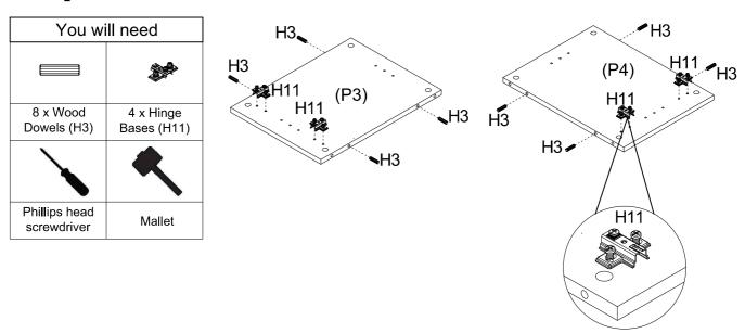
Insert 8 x Wood Dowels (H3) into Side Panels (P3) & (P4). Attach 4 x Hinge Bases (H11) to Side Panels, tighten all screws with a phillips head screwdriver.
