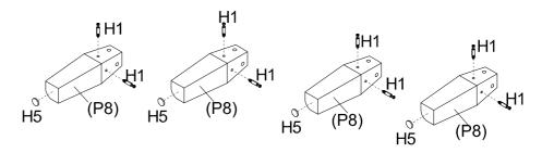
Screw 2 x Cam Bolts (H1) into each Leg (P8) using a phillips head screwdriver.
