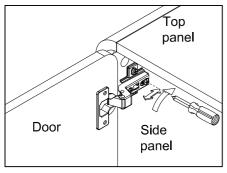
Loosen the screw indicated a little, adjust the hinge to right position (see step 2a & 2b), then tighten the screw.
