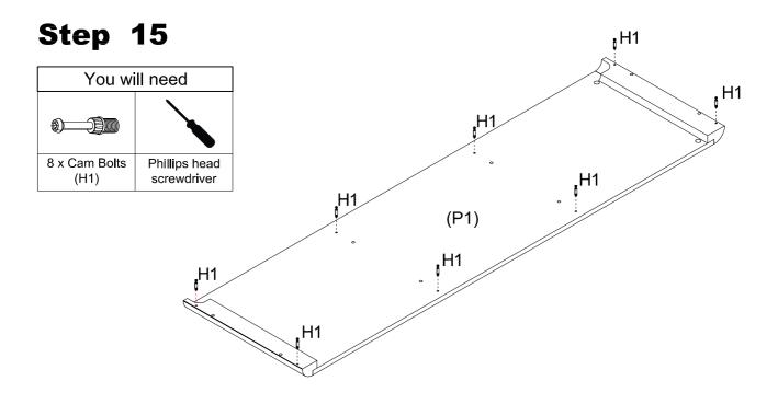
Screw 8 x Cam Bolts (H1) into Top Panel (P1) as shown.
