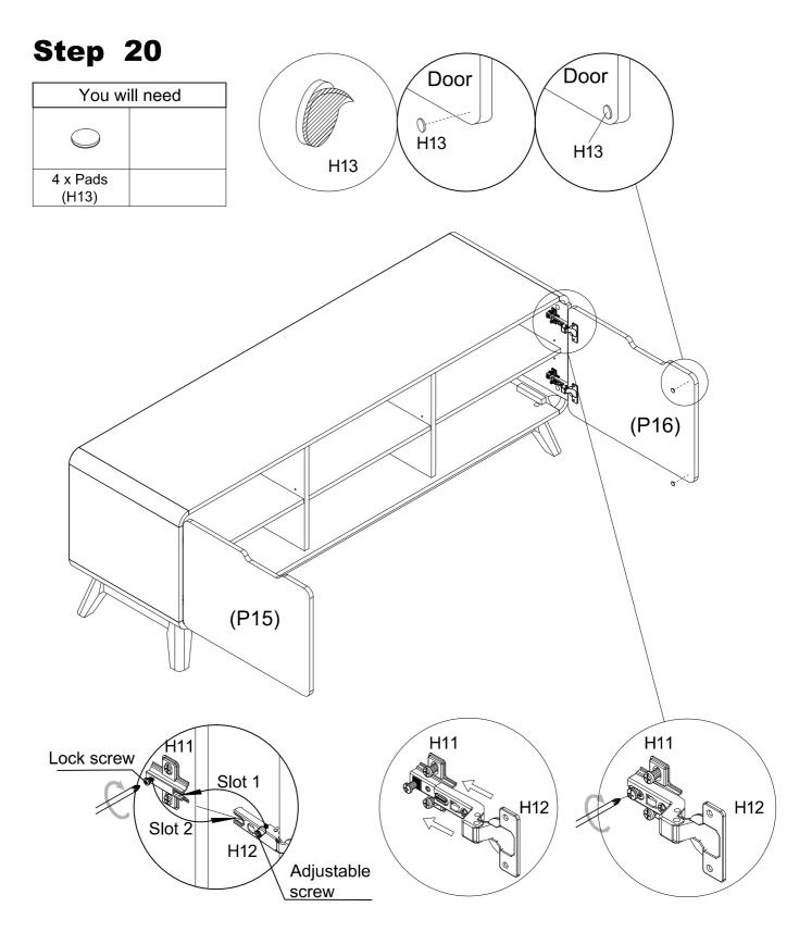
Attach doors onto cabinet as shown. Slide Hinge (H12) onto Hinge Base (H11), until each adjustable screw is in slot 1 and the lock screw is in the slot 2, then tighten lock screw. Attach  $4 \times Pads$  (H13) onto Doors (P15) and (P16).
