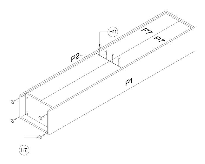
Secure Back Panels (P7x2) to Centre Shelf Panel (P4) with 4 x Nails (H11) along the pre-drawn guideline with the Hammer. Ensure the Nails are evenly spaced along the guideline, approximately 8cm apart. Secure 4 x Feet Glides (H7) to the bottom of Left & Right Side Panels (P1&P2) with the Hammer. Ensure the Feet Glides are evenly spaced, approximately 2cm from the end of each panel.
