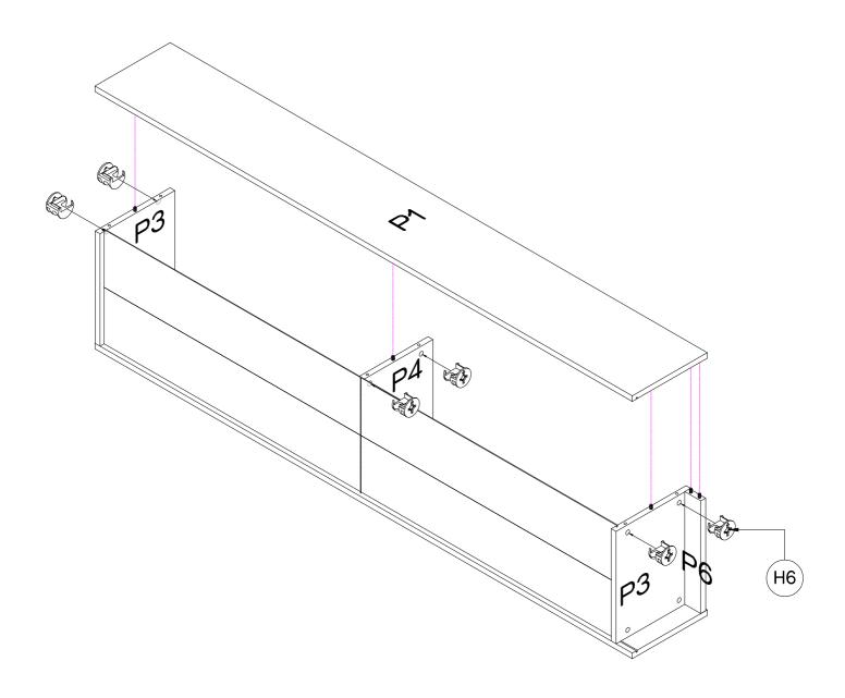
Insert 4 x Cam Nuts (H6) into Top/Bottom Panels (P3x2) and 2 x Cam Nuts (H6) into Centre Panel (P4) as shown. Rotate the cam nuts so the arrows point towards the incoming cam bolts. Secure the Left Side Panel (P1) to Top/Bottom Panels (P3x2) and Centre Panel (P4) by tightening cam nuts with a Phillips Head Screwdriver.
