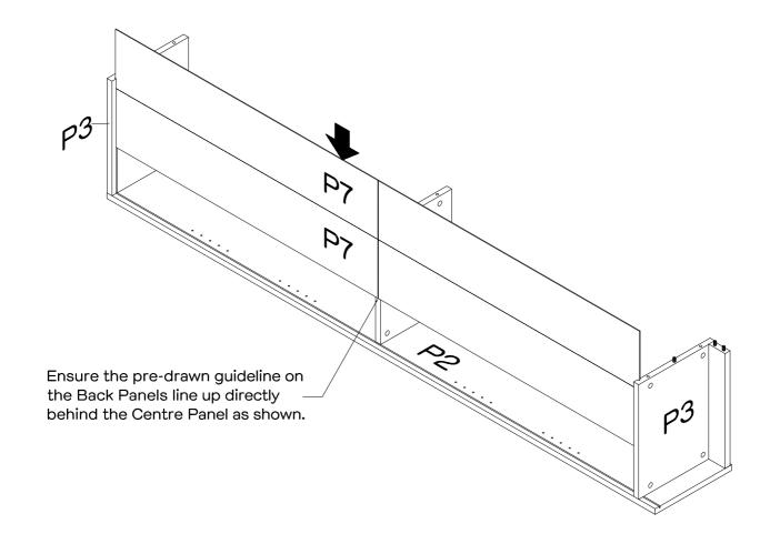
Slide Back Panels (P7x2) into the grooves of Right Side Panel (P2) and Top/Bottom Panels (P3x2) as shown.
