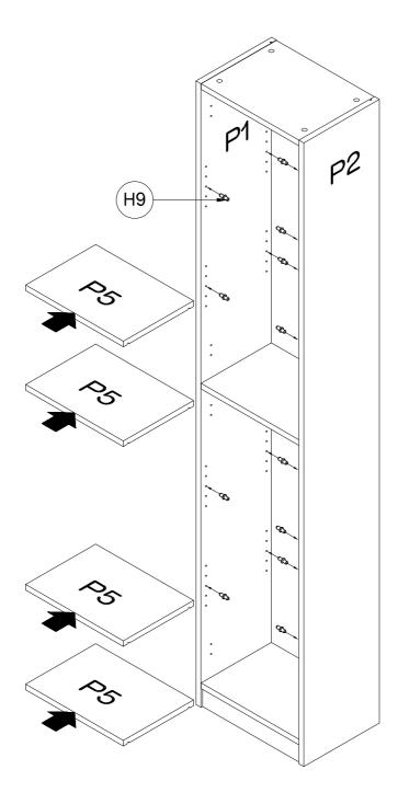
Insert 16 x Shelf Studs (H9) into the Left & Right Side Panels (P1&P2) at your preferred height. Place the Shelf Panels (P5x4) into the unit by resting each shelf on the shelf studs. Ensure each shelf is positioned securely.
