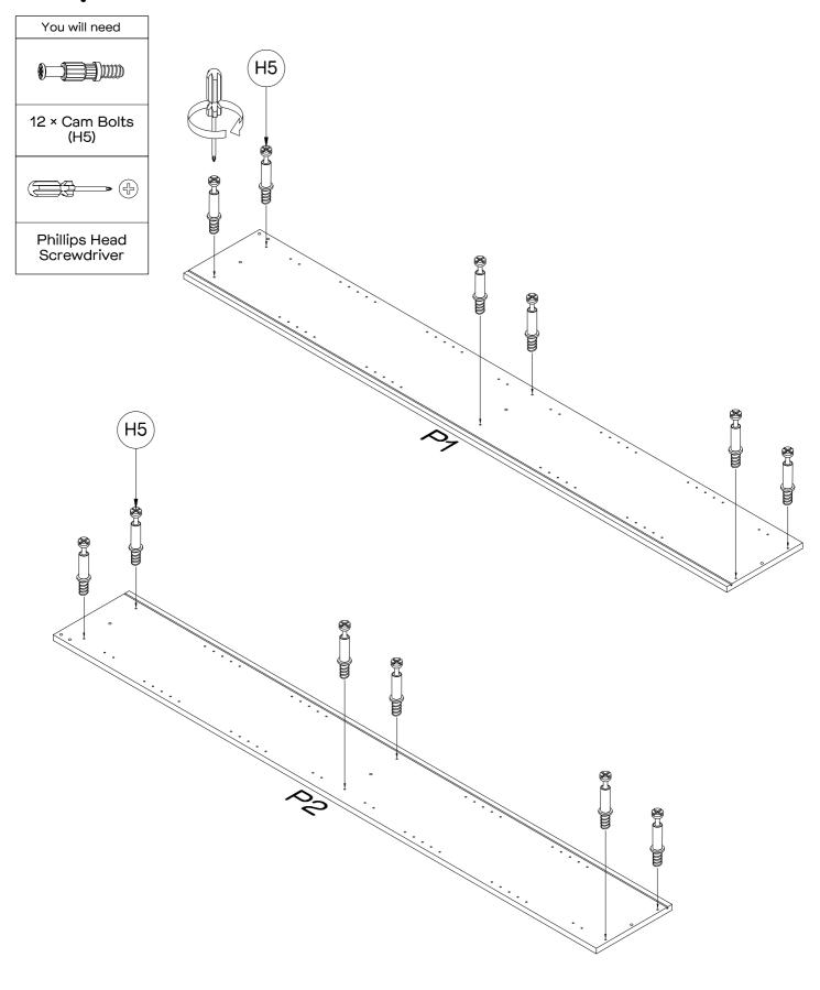
Secure  $6 \times Cam$  Bolts (H5) to Left Side Panel (P1) and  $6 \times Cam$  Bolts (H5) to Right Side Panel (P2) by tightening with the Phillips Head Screwdriver.
