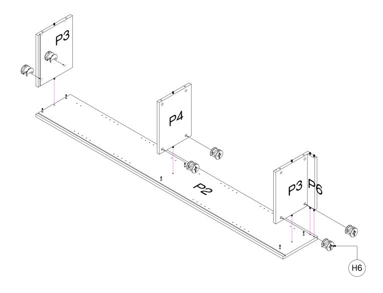
Insert 4 x Cam Nuts (H6) into Top/Bottom Panels (P3x2) and 2 x Cam Nuts (H6) into Centre Panel (P4) as shown. Rotate the cam nuts so the arrows point towards the incoming cam bolts. Secure the Right Side Panel (P2) to Top/Bottom Panels (P3x2) and Centre Panel (P4) by tightening cam nuts with a Phillips Head Screwdriver. Insert Front Panel (P6) into Right Side Panel (P2) as shown.
