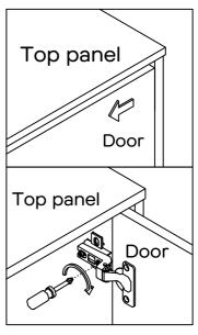
Turn the screw counterclockwise a little as shown to make the gap small.
