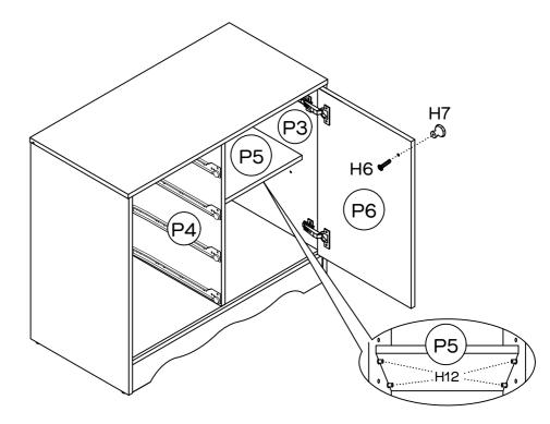
Attach the handle (H7) to panel (P6) with  $1 \times 22$ mm screw (H6) using a phillips head screwdriver.
