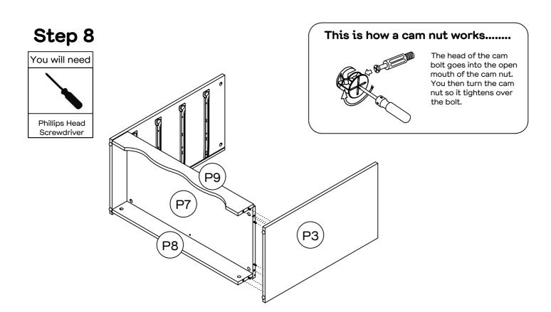
Attach panel (P3) to panels (P7), (P8) & (P9). Turn the cam nut on panels (P7), (P8) & (P9) clockwise motion with a phillips head screwdriver to lock in position.
