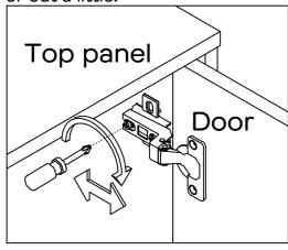
Loosen the screw indicated a little, adjust the hinge to right position, then tighten the screw.
