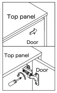
Turn the screw clockwise a little as shown to make the gap big.
