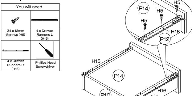
Attach the drawer runner L (H15) and the drawer runner R (H16) to the underside of the drawer with 6 x 12mm screws (H5) using a phillips head screwdriver. Repeat this process for the other 3 drawers.
