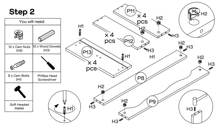
Insert 12 x cam nuts (H2) into panels (P8), (P9), (P11) & (P12). Rotate the cam nuts so the arrows point towards the incoming bolt.
