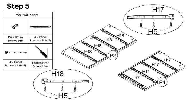
Attach 4 x panel runners R (H17) to the right side panel (P4) with 3 x 12mm screws (H5) using a phillips head screwdriver.
