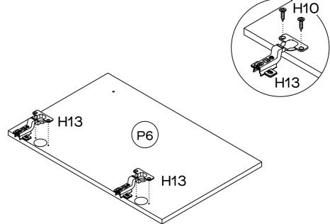
Attach 2 x hinges (H13) to door panel (P6) with  $4 \times 16$ mm screws (H10) using a phillips head screwdriver.
