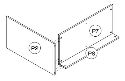
Attach panels (P7), (P8) to panel (P2) by aligning the dowels & cam bolts with the corresponding holes.
