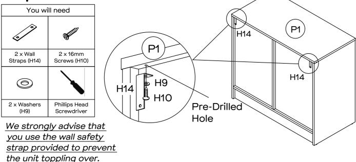
Attach wall fixing strap to panel (P1) with  $2 \times 16$ mm screws (H10) and  $2 \times 4$  washers (H9) using a phillips head screwdriver.
