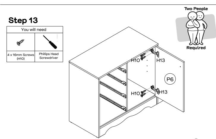
Attach the door (P6) to side panel (P3) by attaching the hinges to panel (P3) with  $4 \times 16$ mm screws (H10) using a philips head screwdriver.
