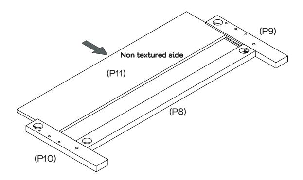
Slide back panel (P11) into the grooves of rails (P8, P9, P10).
