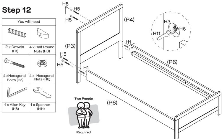
Insert 2 x dowels (H1) into 2 x side rails (P6). Push the 4 x hexagonal bolts (H5) through rails (P3, P4). Attach rails (P3, P4) to 2 x side rails (P6), secure using 4 x hexagonal nuts (H6) and  $4 \times 1$  x half round nuts (H3) with spanner (H11). Tighten  $4 \times 1$  hexagonal bolts (H5) with allen key (H8).
