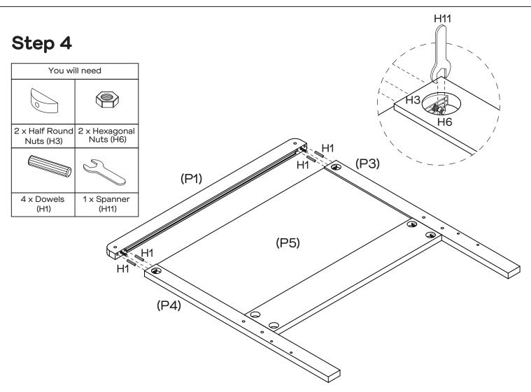
Insert 4 x dowels (H1) into rails (P3, P4). Attach rail (P1) to rails (P3, P4) and secure using 2 x half round nuts (H3) and 2 x hexagonal nuts (H6), tightening with spanner (H11). Ensure that back panel (P5) is slotted into rail (P1).
