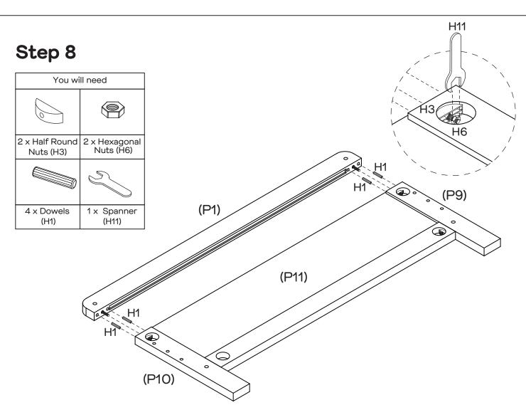
Insert 4  $\times$  dowels (H1) into rails (P9, P10). Attach rail (P1) to rails (P9, P10) and secure using 2  $\times$  half round nuts (H3) and 2  $\times$  hexagonal nuts (H6), tightening with spanner (H11). Ensure that back panel (P11) is slotted into rail (P1).
