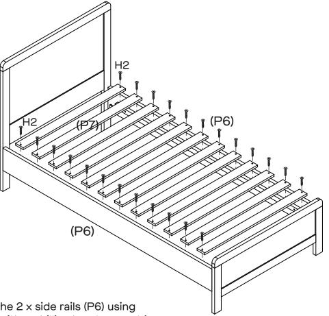
Attach the 12 x slats (P7) to the 2 x side rails (P6) using  $24 \times \text{screws}$  (H2), tightening with a phillips head screwdriver.
