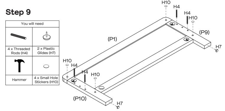
Attach 4 x threaded rods (H4) into rails (P9, P10). Attach 2 x plastic glides (H7) to the end of rails (P9, P10) by gently tapping with a hammer. Attach 4 x small hole stickers (H10) to the holes of rails (P1, P9, P10).
