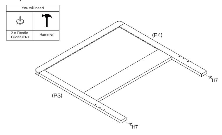
Attach 2 x plastic glides (H7) to the end of rails (P3, P4) by gently tapping with a hammer.
