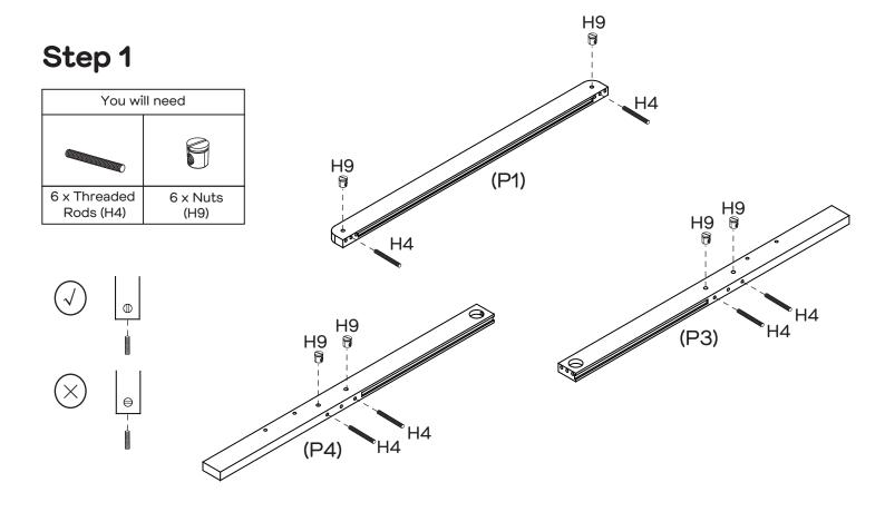
Insert 6 x nuts (H9) into the holes in rails (P1, P3, P4). Ensure the lines in the nuts (H9) face incoming threaded rods as shown in the image above. Attach 6 x threaded rods (H4) to the 6 x nuts (H9) and hand tighten by turning clockwise.
