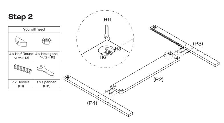
Insert 2 x dowels (H1) into rail (P2). Attach rails (P3, P4) to rail (P2) and secure using 4 x half round nuts (H3) and 4 x hexagonal nuts (H6), tightening with spanner (H11).
