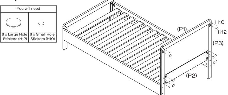
Cover the holes on rails (P2, P3, P4) using 6 x large hole stickers (H12). Cover the holes on rails (P1, P3, P4) using 6 x small hole stickers (H10).
