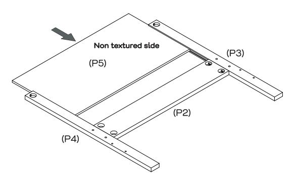
Slide back panel (P5) into the grooves of rails (P2, P3, P4).
