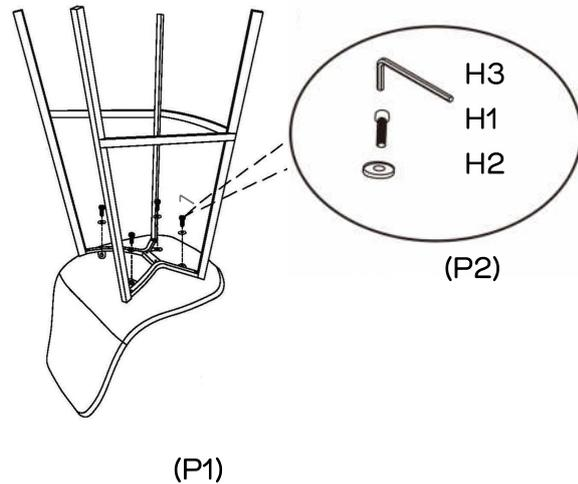
Align the holes on the frame (P2) to the holes on the seat (P1)
