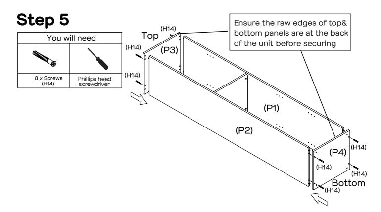
Attach Top & Bottom Panels (P3&P4) to Left & Right Side Panels (P1&P2) as shown with 8 x Screws (H14) by tightening with the Phillips Head Screwdriver.
