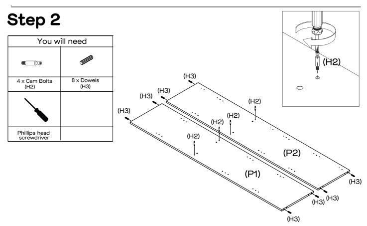
Attach 4 x Cam Bolts (H2) to Left & Right Side Panels (P1 & P2) as shown by tightening with the Phillips Head Screwdriver.Insert 8 x Dowels (H3) into Left & Right Side Panels (P1 & P2).
