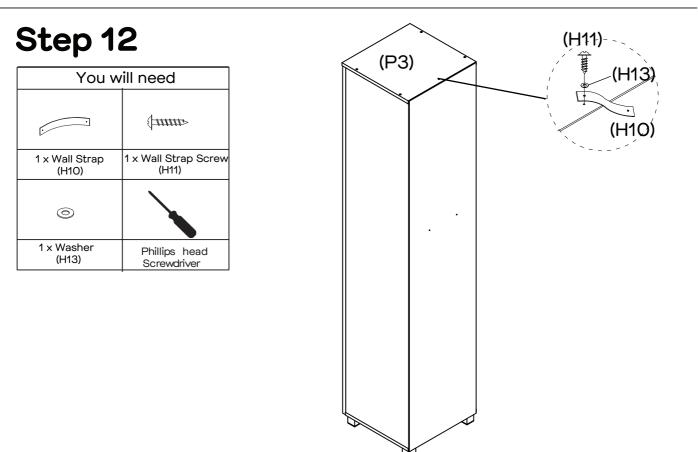
Attach Wall Strap (H10) to Top Panel (P3) with 1 x Washer (H13) and 1 x Wall Strap Screw (H11) as shown by tightening with the Phillips Head Screwdriver.
