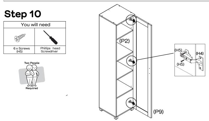
With assistance carefully align the 3 x Hinges (H4) on the Door (P9) to Right Side Panel (P2) and secure with 6 x Screws (H5) by tightening with the Phillips Head Screwdriver.
