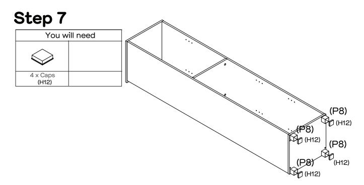
Attach 4 x Caps (H12) to Feet (P8x4) by pressing firmly into place. Ensure they are secured well.
