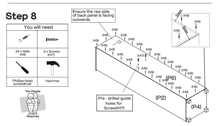
Align Back Panel (P6) with the edges of the partially assembled unit and the pre-drilled holes with the back of the fixed shelf. Attach Back Panel (P6) to the back of Fixed Shelf (P5) with 2 x Screws (H17) by tightening with the Phillips Head Screwdriver. Attach Back Panel (P6) to Left, Right, Top&Bottom Panels (P1, P2, P3&P4) with 34 x Nails (H9) with the Hammer. Ensure the nails are evenly spaced out as shown and are placed approximately 5mm from the edge of the back panel.
