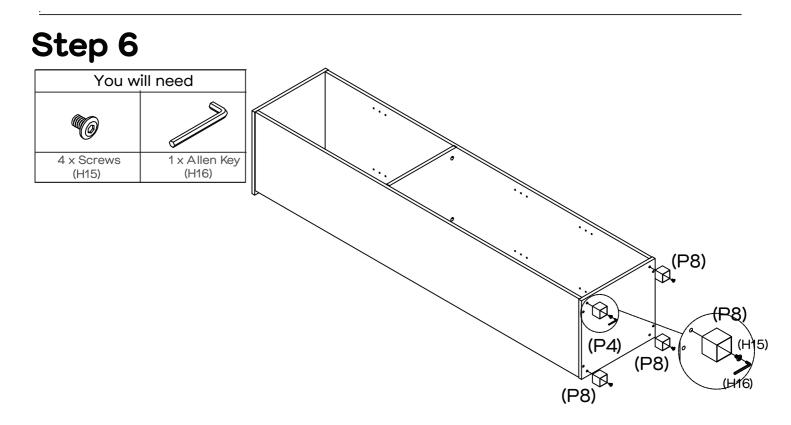
Attach Feet (P8x4) to Bottom Panel (P4) with  $4 \times$  Screws (H15) by tightening with the Allen Key (H16).
