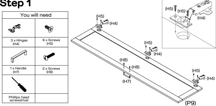
Attach 3 x Hinges (H4) to Door (P9) as shown with 6 x Screws (H5) by tightening with the Phillips Head Screwdriver. Secure 1 x Handle (H7) to the front of Door (P9) with 2 x Screws (H8) by tightening with the Phillips Head Screwdriver.
