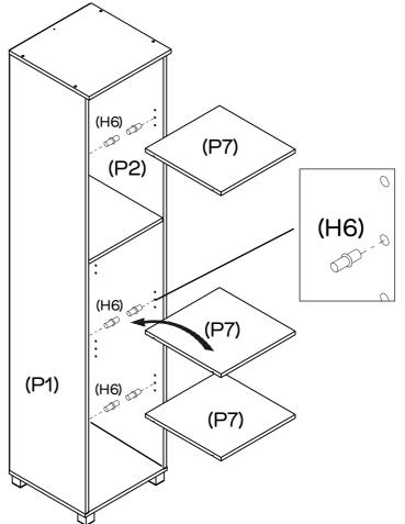
Insert 12 x Shelf Supports (H6) to Left & Right Side Panels (P1&P2) as shown at your desired height. Place Adjustable Shelves (P7x3) into the unit and rest on shelf supports. Ensure the shelves are firmly secured.
