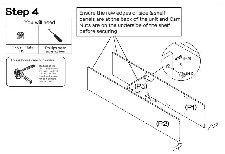
Insert 4 x Cam Nuts (H1) into Fixed Shelf (P5).Rotate the Cam Nuts so the arrows point towards the incoming cam bolts.Attach Left & Right Side Panels (P1&P2) to Fixed Shelf (P5) by tightening the Cam Nuts with the Phillips Head Screwdriver.
