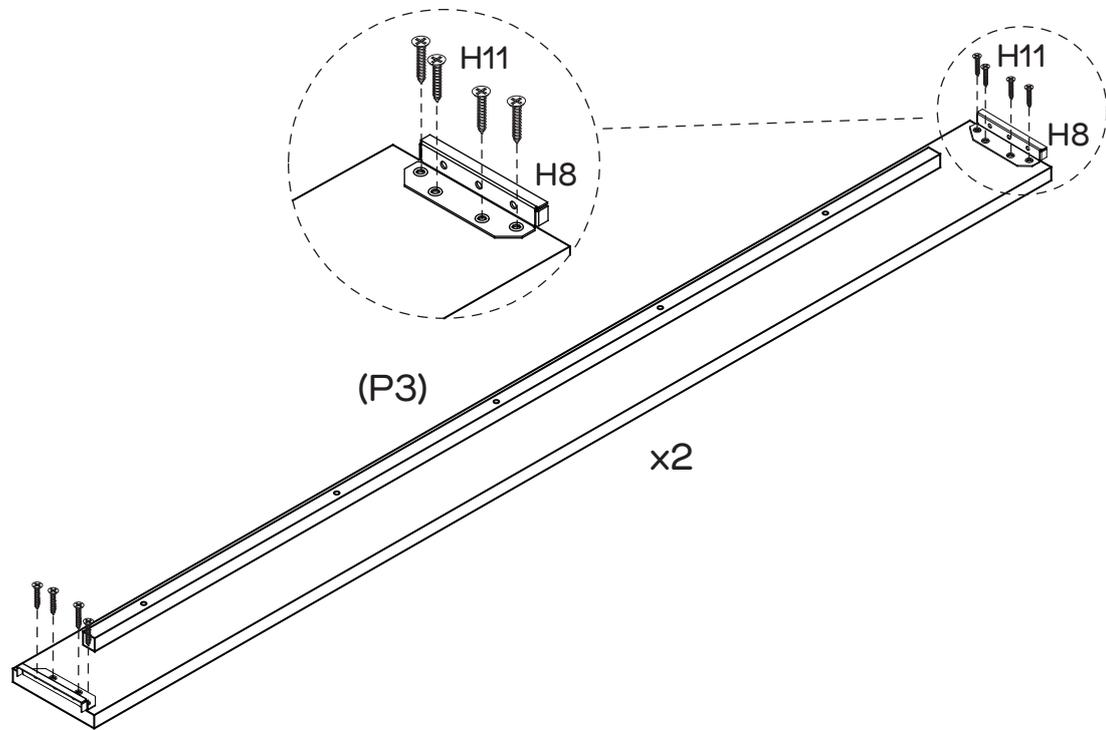
Attach 4 x elbow connectors (H8) to the ends of the 2 x side panels (P3) with 16 x screws (H11), tightening with a phillips head screwdriver.
