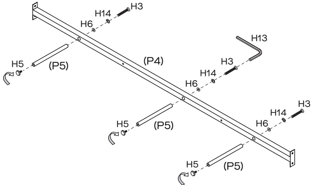
Attach 3 x support legs (P5) to centre rail (P4) using 3 x washers (H6), 3 x spring washers (H14) and 3 x long bolts (H3), tightening with the allen key (H13). Attach the 3 x adjusters (H5) to the 3 x support legs (P5) by turning clockwise.
