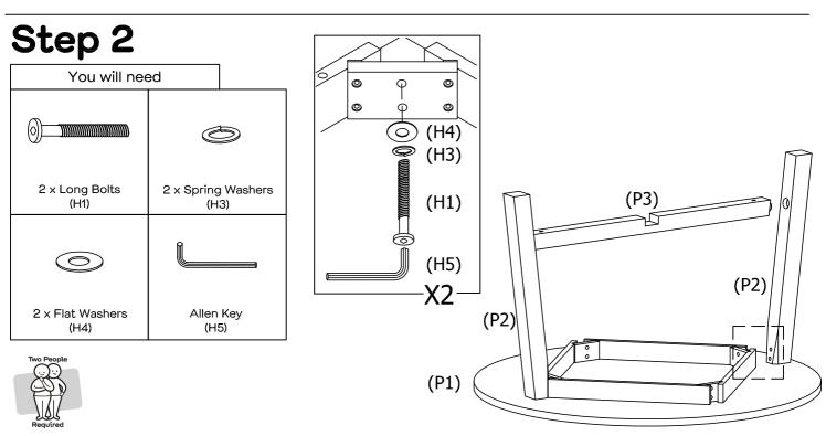
Slot 1 x bottom stretcher (P3) into the table leg (P2) attached to the table top (P1). Slot the other end of the bottom stretcher (P3) into 1 x table leg (P2) and secure the table leg (P2) to the table top (P1) with 2 x long bolts (H1), 2 x spring washers (H3) and 2 x flat washers (H4) using allen key (H5). Do not fully tighten the bolts until Step 5.
