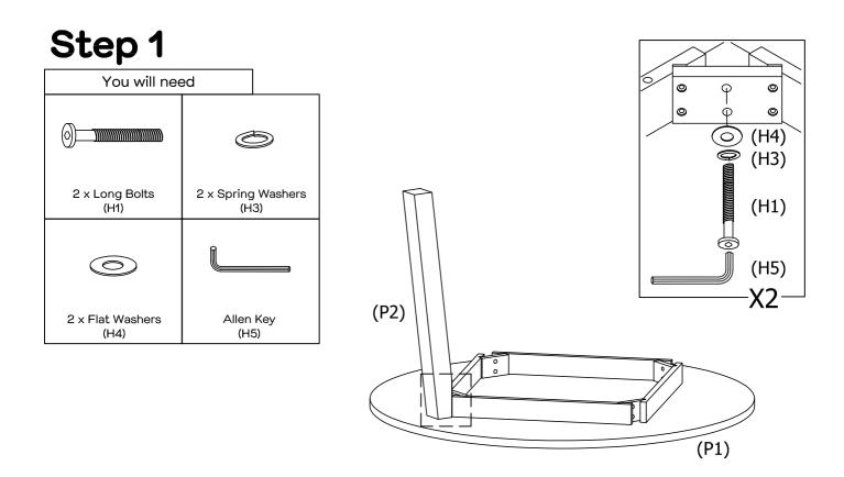
Attach 1 x table leg (P2) to table top (P1) with 2 x long bolts (H1), 2 x spring washers (H3) and 2 x flat washers (H4) using allen key (H5). Do not fully tighten the bolts until Step 5.
