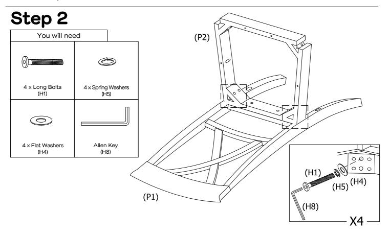
Further secure seat frame (P2) to chair back (P1) using  $4 \times 1000$  bolts (H1),  $4 \times 1000$  spring washers (H5) and  $4 \times 1000$  fully tighten the bolts until Step 6.
