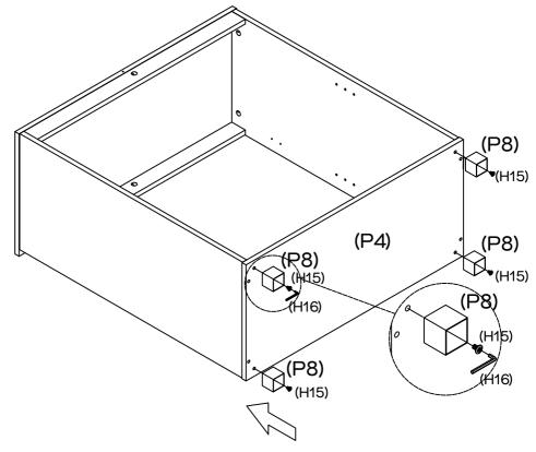
Attach Feet (P8x4) to Bottom Panel (P4) with 4 x Screws (H15) by tightening with the Allen Key (H16).
