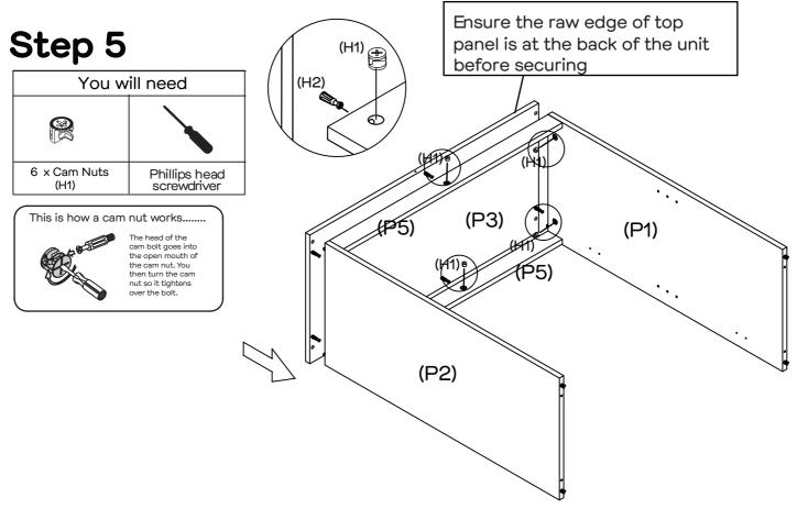
Insert 6 x Cam Nuts (H1) into Left & Right Side Panels (P1&P2) and Support Panels (P5 x 2) as shown. Rotate the Cam Nuts so the arrowspoint towards the incoming cam bolts. Attach Top Panel (P3) to Left & Right Side Panels (P1&P2) and Support Panels (P5 x 2) by tightening the Cam Nuts with the Phillips Head Screwdriver.
