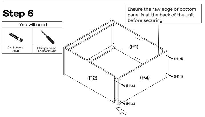
Attach Bottom Panel (P4) to Left & Right Side Panels (P1&P2) with 4 x Screws (H14) by tightening with the Phillips Head Screwdriver.
