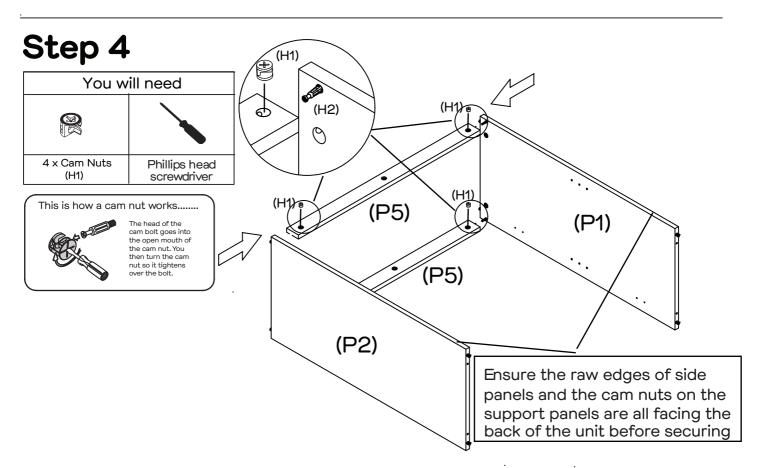
Insert 4 x Cam Nuts (H1) into Support Panels (P5 x 2). Rotate the Cam Nuts so the arrows point towards the incoming cam bolts. Attach Left & Right Side Panels (P1&P2) to Support Panels (P5 x 2) by tightening the Cam Nuts with the Phillips Head Screwdriver.
