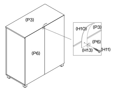
Attach Wall Strap (H10) to Top Panel (P3) with  $1 \times \text{Washer}$  (H13) and  $1 \times \text{Wall}$  Strap Screw (H11) as shown by tightening with the Phillips Head Screwdriver.
