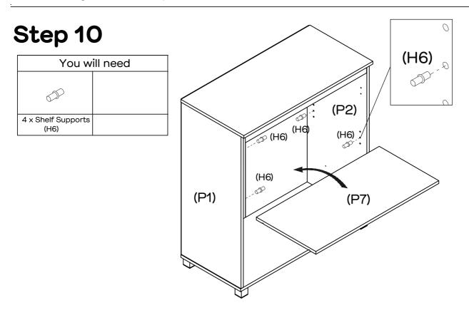
Insert 4 x Shelf Supports (H6) into Left & Right Side Panels (P1&P2) as shown at your desired height. Place Adjustable Shelf (P7) into the unit and rest on shelf supports. Ensure the shelves are firmly secured.
