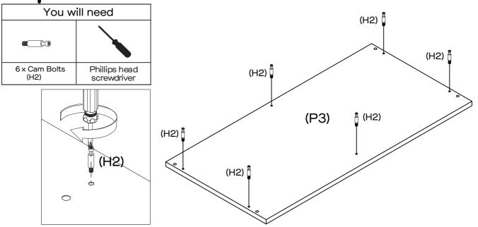
Attach 6 x Cam Bolts (H2) to Top Panel (P3) by tightening with the Phillips Head Screwdriver.
