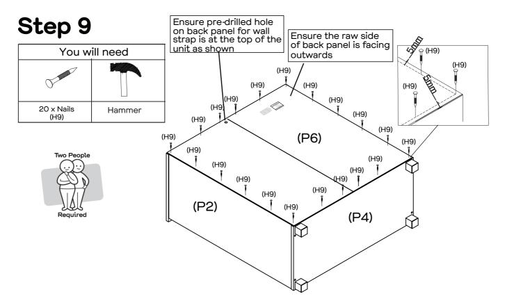
Align the Back Panel (P6) with the edges of the partially assembled unit. Attach Back Panel (P6) to Left,Right,Top&Bottom Panels (P1,P2,P3&P4) with 20 x Nails (H9) with the Hammer.Ensure the nails are evenly spaced out as shown an are placed approximately 5mm from the edge of the back panel.
