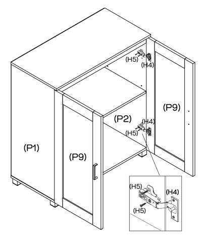
With assistance carefully align the 2 x Hinges (H4) on the Door (P9) to Right Side Panel (P2) and secure with 4 x Screws (H5) by tightening with the Phillips Head Screwdriver. Repeat steps for the second Door (P9).
