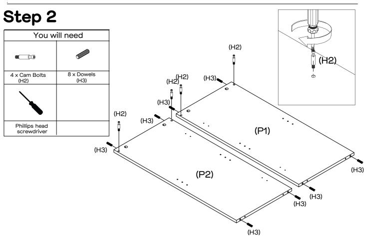
Attach 4 x Cam Bolts (H2) to Left & Right Side Panels (P1 & P2) as shown by tightening with the Phillips Head Screwdriver. Insert 8 x Dowels (H3) into Left & Right Side Panels (P1 & P2).
