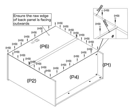
Carefully align the edges of the Back Panel (P6) with the frame of the partially assembled unit. Secure Back Panel (P6) to Bottom Panel (P4),Top Panel (P3), and Left & Right Side Panels (P1&P2) with 32 x Nails (H9) as shown using the Hammer. Fix each nail 5mm from the edge of the Back Panel (P6).
