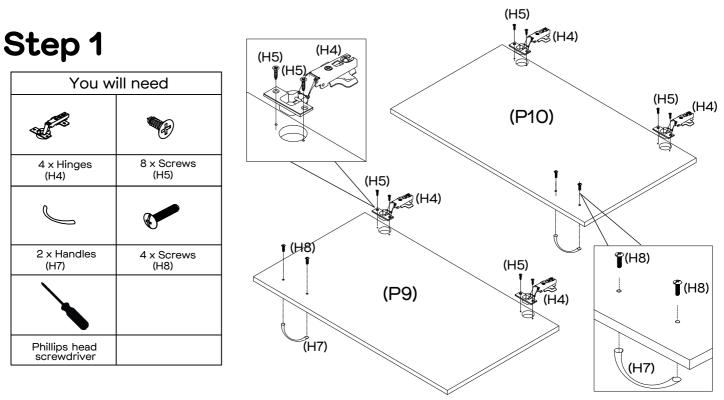
Attach 4 x Hinges (H4) to Left & Right Door Panels (P9&P10) as shown with 8 x Screws (H5) by tightening with the Phillips Head Screwdriver.
