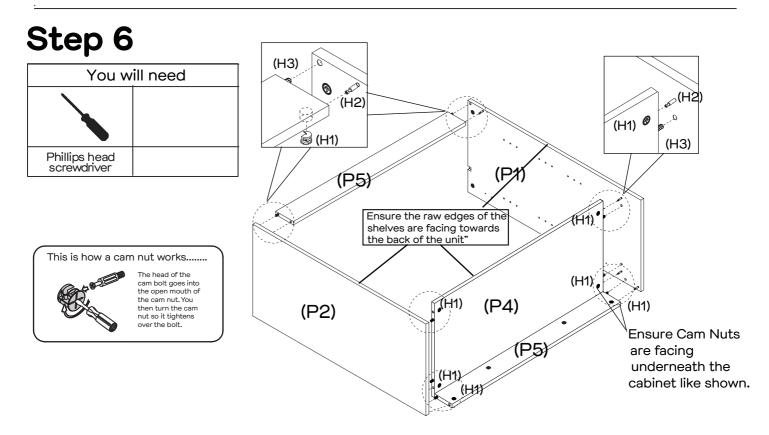
Attach Bottom Panel (P4) and Support Panels (P5x2) to Left & Right Side Panels (P1&P2) and secure by tightening all 8 x Cam Nuts (H1) with the Phillips Head Screwdriver.
