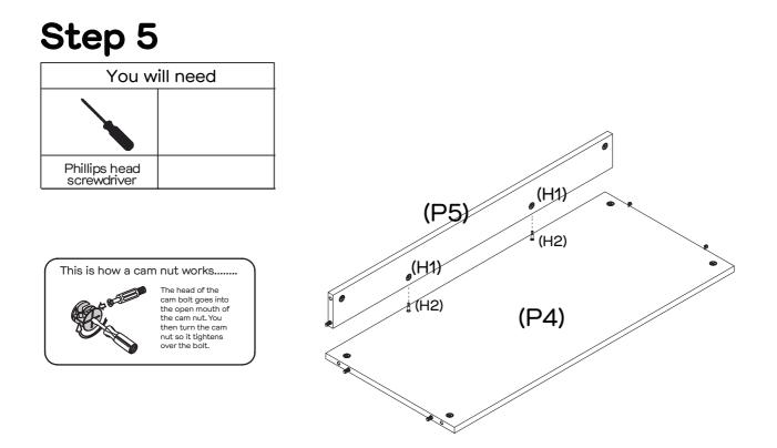
Attach Support Panel (P5) to Bottom Panel (P4) by tightening  $2 \times Cam$  Nuts (H1) with the Phillips Head Screwdriver.
