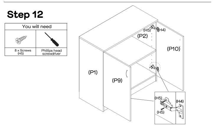
Secure 4 x Hinges (H4) on Left & Right Door Panels (P9&P10) to Left & Right Side Panels (P1&P2) with 8 x Screws (H5) as shown by tightening with the Phillips Head Screwdriver.
