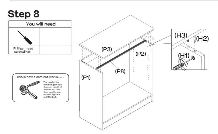
Place the Steel Bar (P8) into the grooves of Left & Right Side Panels (P1&P2). Align the Top Panel (P3) with Support Panel (P5) and Left & Right Side Panels (P1&P2) and attach by tightening the 6 x Cam Nuts (H1).
