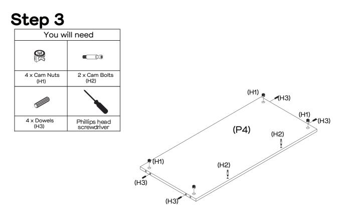
Insert 4 x Dowels (H3) & 4 x Cam Nuts (H1) into Bottom Panel (P4) as shown. Attach 2 x Cam Bolts (H2) to Bottom Panel (P4) by tightening with the Phillips Head Screwdriver.
