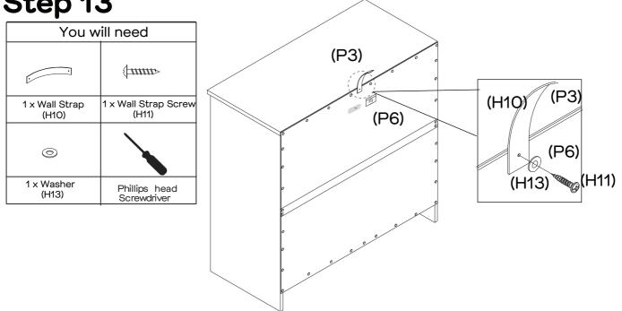
Attach Wall Strap (H10) to the back of Top Panel (P3) with Washer (H13) and Wall Strap Screw (H11) by tightening with the Phillips Head Screwdriver.
