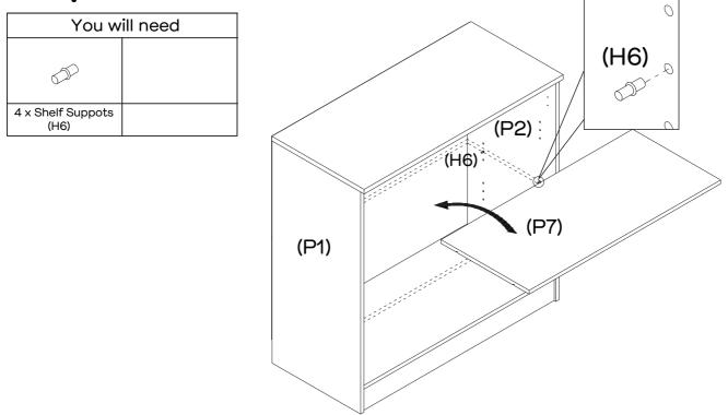
Insert 4 x Shelf Supports (H6) into Left & Right Side Panels (P1&P2) at your preferred height. Place Shelf Panel (P7) into the assembled unit and gently rest on the Shelf Supports. Ensure that the Shelf is firmly secured.
