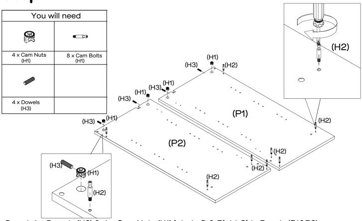
Insert 4 x Dowels (H3) & 4 x Cam Nuts (H1) into Left & Right Side Panels (P1&P2) as shown. Attach 8 x Cam Bolts (H2) to Left & Right Side Panels (P1&P2) by tightening with the Phillips Head Screwdriver. Fantastic furniture.com.au
