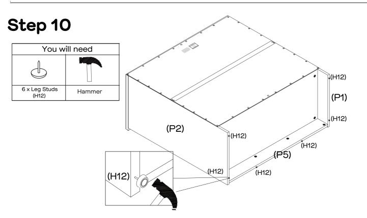
Secure 6 x Leg Studs (H12) to Support Panel (P5) and Left & Right Side Panels (P1&P2) as shown using the Hammer.
