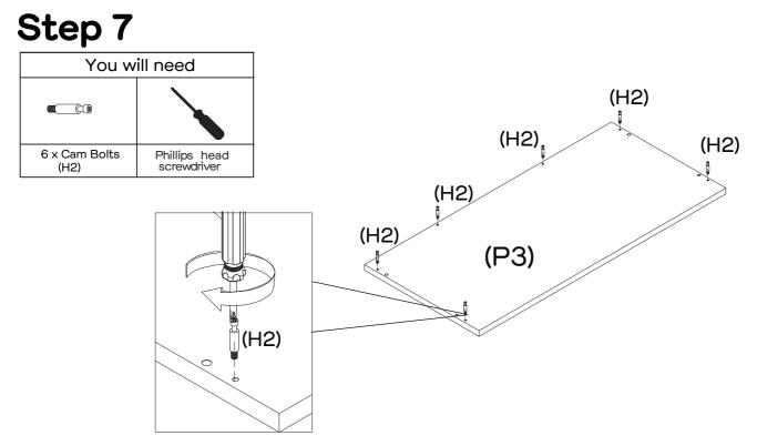
Attach 6 x Cam Bolts (H2) to Top Panel (P3) by tightening with the Phillips Head Screwdriver.
