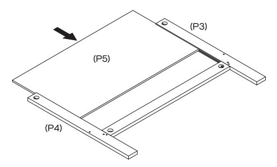
Slide back panels (P5) into the grooves of rails (P3, P4).
