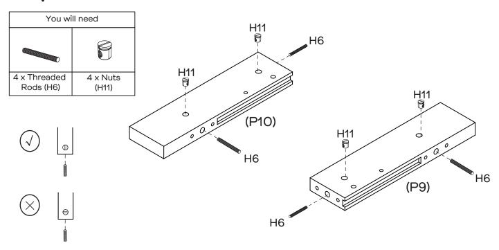
Insert 4 x nuts (H11) into the holes in rails (P9, P10). Ensure the lines in the nuts (H11) face incoming threaded rods as shown in the image above. Attach 4 x threaded rods (H6) to the  $4 \times 1$  nuts (H11) and hand tighten by turning clockwise.
