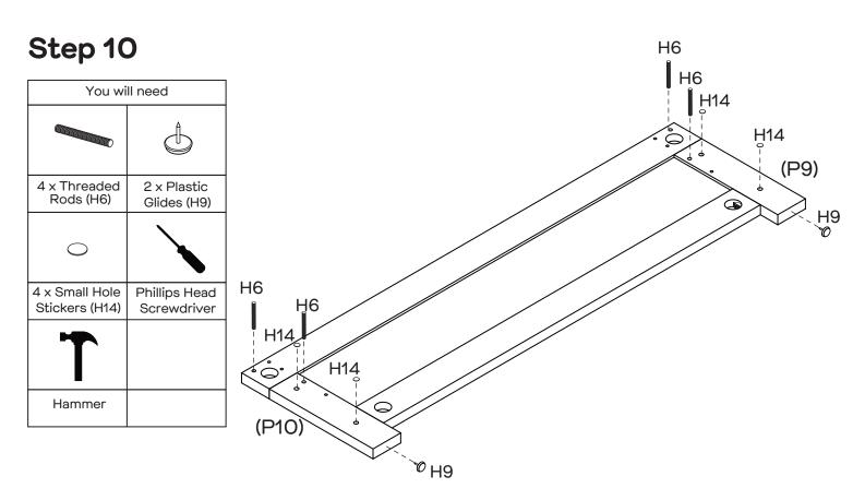
Attach 4 x threaded rods (H6) into rails (P9, P10). Attach 2 x plastic glides (H9) to the end of rails (P9, P10) by gently tapping with a hammer. Attach 4 x small hole stickers (H14) to the holes of rails (P9, P10).
