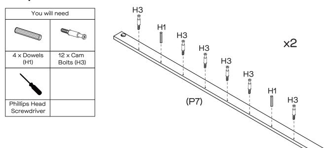
Insert 2 x dowels (H1) into the side cover (P7). Attach 6 x cam bolts (H3) into 1 x side cover (P7), tightening with a phillips head screwdriver.
