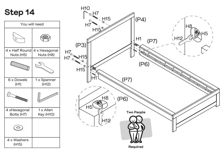
Insert 6 x dowels (H1) into 2 x side covers (P7) and 2 x side rails (P6). Thread 4 x hexagonal bolts (H7) through the 4 x washers (H15) and push the 4 x hexagonal bolts (H7) through rails (P3, P4). Attach rails (P3, P4) to 2 x side covers (P7) and 2 x side rails (P6), secure using 4 x hexagonal nuts (H8) and 4 x half round nuts (H5) with spanner (H12). Tighten 4 x hexagonal bolts (H7) with allen key (H10).
