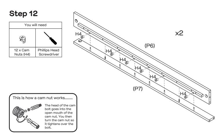
Insert 6 x cam nuts (H4) into the holes on the side rail (P6). Rotate the cam nuts so the arrows point towards the incoming cam bolts. Attach the side rail (P6) to the side cover (P7), then tighten the cam nuts with a phillips head screwdriver. Repeat step 11 and step 12 for the other side cover (P7) and side rail (P6).
