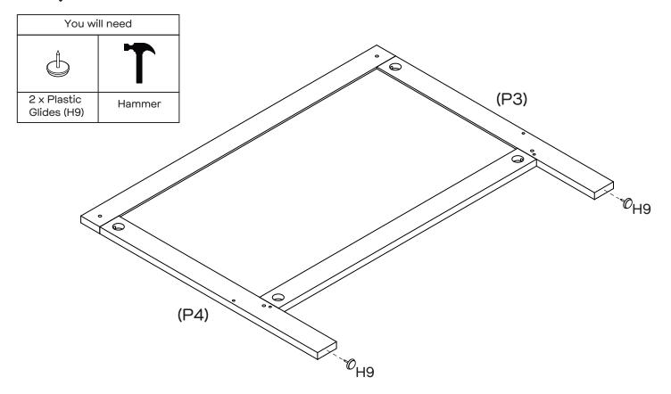
Attach 2 x plastic glides (H9) to end of rails (P3, P4) by gently tapping with a hammer.
