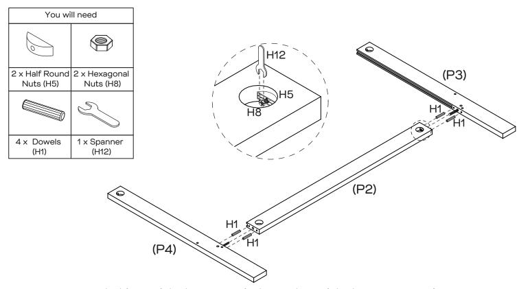
Insert 4 x dowels (H1) into rail (P2). Attach rails (P3, P4) to rail (P2) and secure using  $2 \times 1$  x half round nuts (H5) and  $2 \times 1$  x hexagonal nuts (H8), tightening with spanner (H12).
