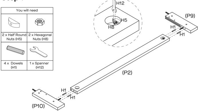
Insert 4 x dowels (H1) into rail (P2). Attach rails (P9, P10) to rail (P2) and secure using 2 x half round nuts (H5) and 2 x hexagonal nuts (H8), tightening with spanner (H12).
