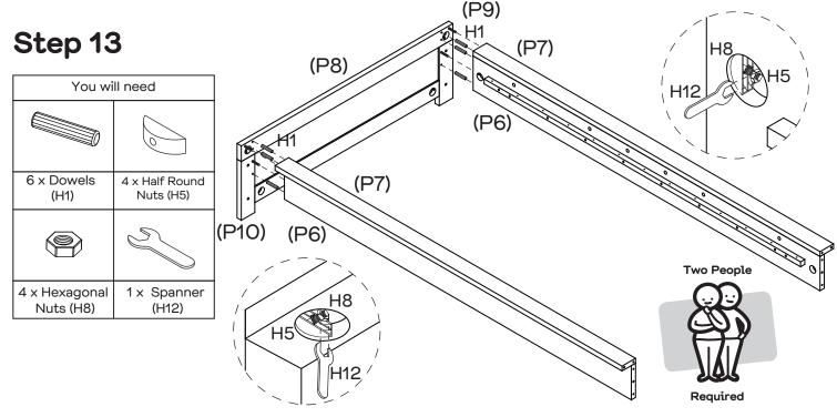
Insert 6 x dowels (H1) into 2 x side covers (P7) and 2 x side rails (P6). Attach rails (P9, P10) to 2 x side covers (P7) and 2 x side rails (P6) and secure using 4 x hexagonal nuts (H8) and 4 x half round nuts (H5), tightening with the spanner (H12).
