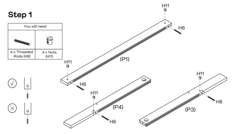
Insert 4 x nuts (H11) into the holes in rails (P1, P3, P4). Ensure the lines in the nuts (H11) face incoming threaded rods as shown in the image above. Attach 4 x threaded rods (H6) to the  $4 \times 1$  nuts (H11) and hand tighten by turning clockwise.
