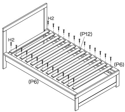
Attach the 13  $\times$  slats (P12) to the 2  $\times$  side rails (P6) using 26  $\times$  screws (H2), tightening with a phillips head screwdriver.
