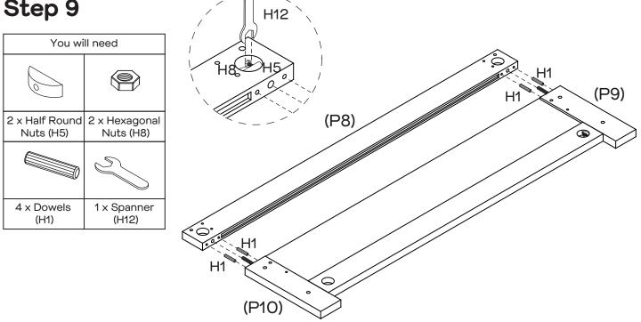
Insert 4 x dowels (H1) into rails (P9, P10). Attach rail (P8) to rails (P9, P10) and secure using 2 x half round nuts (H5) and 2 x hexagonal nuts (H8), tightening with spanner (H12).
