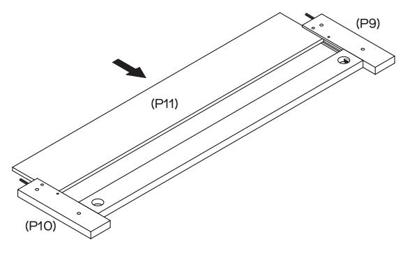
Slide back panel (P11) into the grooves of rails (P9, P10).
