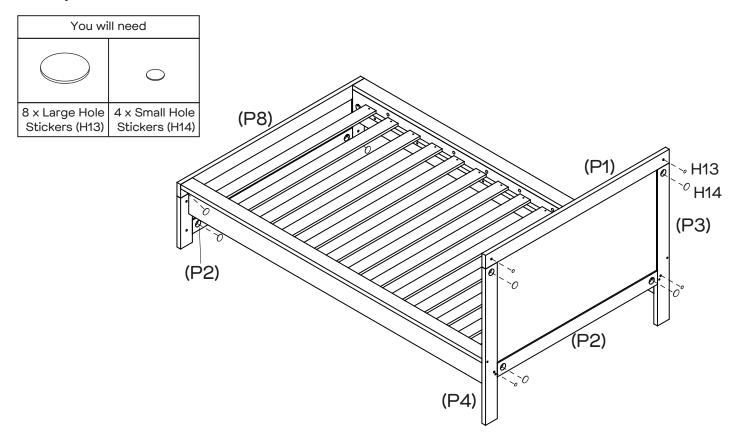
Cover the holes on rails (P2, P3, P4, P8) using 8 x large hole stickers (H13). Cover the holes on rails (P1, P3, P4) using 4 x small hole stickers (H14).
