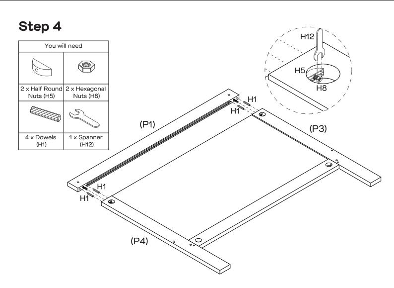
Insert 4 x dowels (H1) into rails (P3, P4). Attach rail (P1) to rails (P3, P4) and secure using  $2 \times 1$  half round nuts (H5) and  $2 \times 1$  hexagonal nuts (H8), tightening with spanner (H12).
