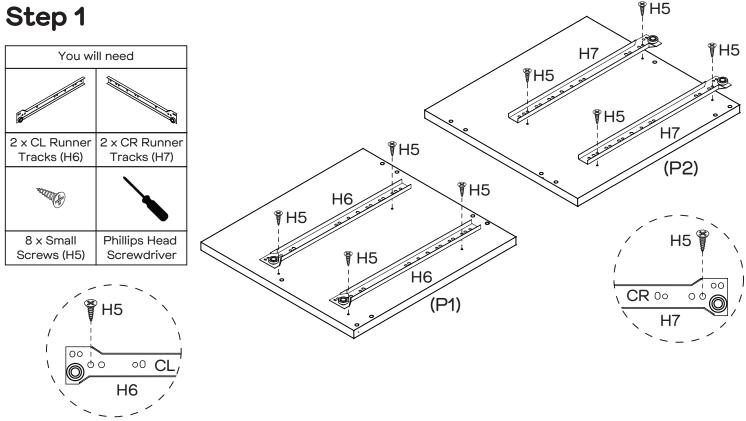
Attach 2 x CL Runner Tracks (H6) to Left Side Panel (P1) with 4 x Small Screws (H5). Attach 2 x CR Runner Tracks (H7) to Right Side Panel (P2) with 4 x Small Screws (H5).
