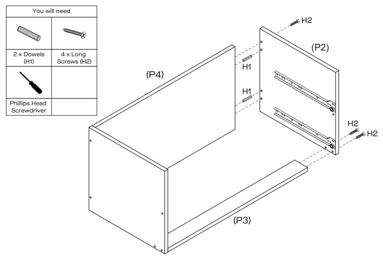
Insert 2 x Dowels (H1) into the holes of Back Panel (P4) as shown. Attach Right Side Panel (P2) to Back Panel (P4) and Rail (P3) with 4 x Long Screws (H2). Tighten the screws with a Phillips Head Screwdriver.
