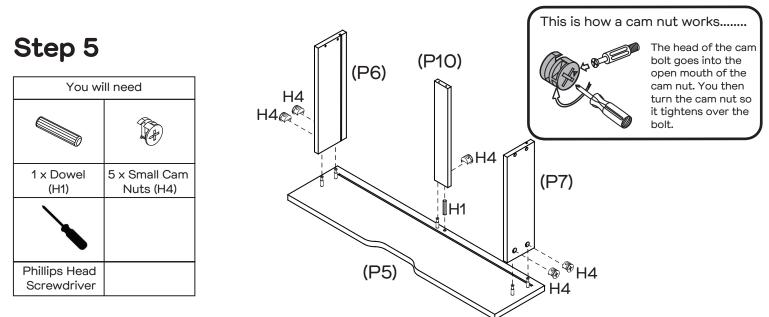
Insert 1 x Dowel (H1) into Drawer Front (P5) as shown.
