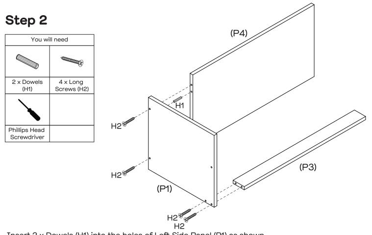
Insert 2 x Dowels (H1) into the holes of Left Side Panel (P1) as shown. Attach Back Panel (P4) and Rail (P3) to Left Side Panel (P1) with 4 x Long Screws (H2) using a Phillips Head Screwdriver.
