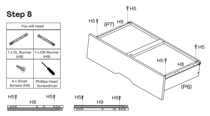
Attach 1 x DL Runner (H8) to the bottom of Left Drawer Side (P6) and 1 x DR Runner (H9) to the bottom of Right Drawer Side (P7) with 4 x Small Screws (H5). Tighten Screws using a Phillips Head Screwdriver.
