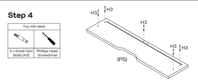
Screw 5 x Small Cam Bolts (H3) into Drawer Front (P5) with a Phillips Head Screwdriver.
