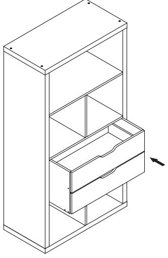
Put the insert cabinet into the bookcase, make sure the drawer front of insert cabinet is flush with the edge of shelf.
