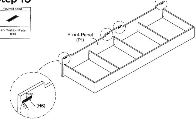
Remove cushion pads from adhesive stickers and paste on front panel (P1). Make sure the cushion pads (H6) do not exceed 3mm from the top panel as shown in picture.
