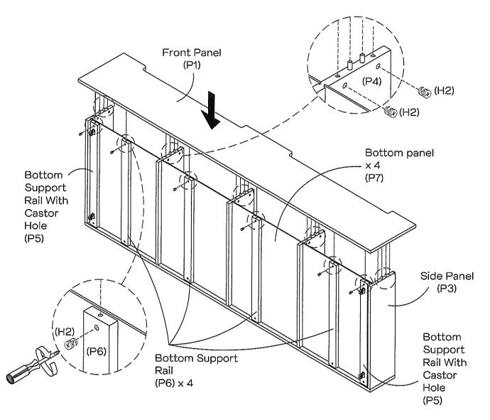
Insert 16 x cam nuts (H2) into the panels (P3, P4, P5 & P6). Rotate the cam nuts (H2) so the arrows point towards the incoming cam bolts. Attach the front panel (P1) to panels (P3, P4, P5, P6 & P7).
