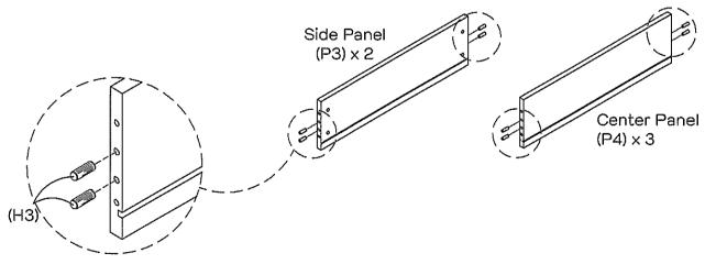
Insert 20 x wood dowels (H3) to the panels as shown by hand or gently using a soft headed mallet.
