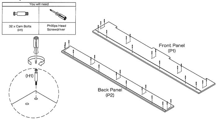
Insert 32  $\times$  cam bolts (H1) into the front panel (P1) and back panel (P2) as shown, tighten with a phillips head screwdriver.
