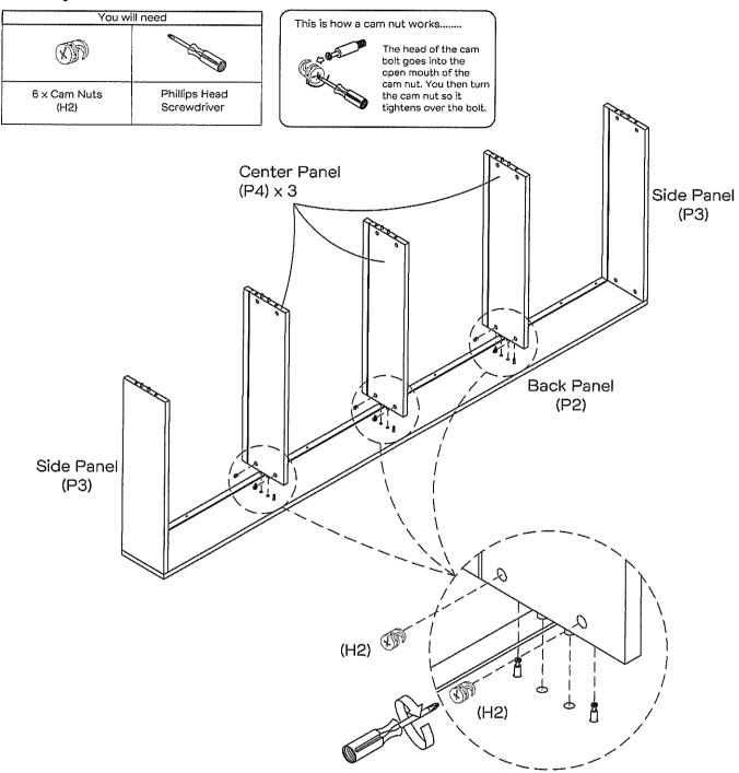
Insert 6 x cam nuts (H2) into center panels (P4).
