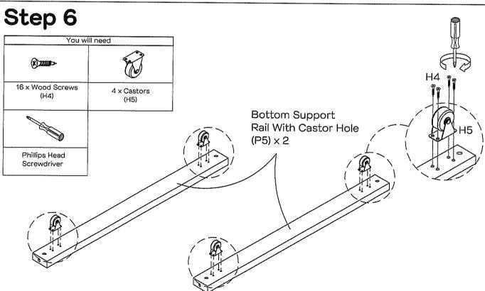
Attach  $4 \times$  castors (H4) to the bottom support rails with castor holes (P5) using  $16 \times$  wood screws (H4) tightening with the phillips head screwdriver.
