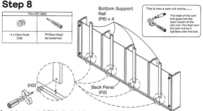
Insert  $4 \times \text{cam}$  nuts (H2) into the  $4 \times \text{bottom}$  support rails (P6). Rotate the cam nuts (H2) so the arrows point towards the incoming cam bolts. Attach the  $4 \times \text{bottom}$  support rails (P6) to the back panel (P2). Turn the cam nuts (H2) on rails (P6) clockwise with a phillips head screwdriver to lock into position.
