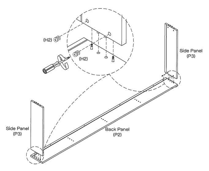
Insert  $4 \times$  cam nuts (H2) into the side panels (P3).
