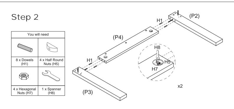
Insert 8 x Dowels (H1) into Rails (P4x2). Attach Legs (P2x2, P3x2) to Rail (P4x2) with 4 x Half Round Nuts (H5), and 4 x Hexagonal Nuts (H7) using Spanner (H8).
