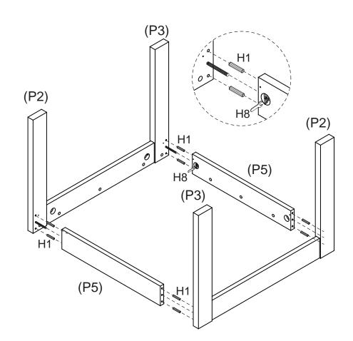
Insert 8 x Dowels (H1) into Rail (P5x2), attach to Legs (P2x2, P3x2). Insert 4 x Half Round Nuts (H5), and 4 x Hexagonal Nuts (H7) using Spanner (H8).
