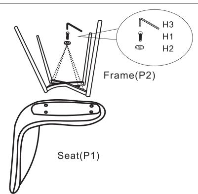
Align the holes on the Frame ( P2 ) to the Screw holes of the seat ( P1 ). Fix Frame ( P2 ) to the Seat ( P1 ) with 4 X Washes ( P2 ) and 4 X Screws ( P1 ). Fully tighten the bolts using Allen Key ( P1 ). Turn the chair over carefully.
