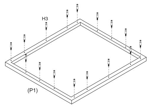
Secure 16 x Cam Bolts (H3) to Top Panel (P1) by tightening Cam Bolts (H3) with a Phillips Head Screwdriver.
