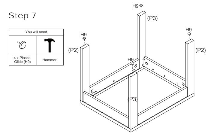
Attach 4 x Plastic Glides (H9) to the Legs (P2x2&P3x2) by using a hammer to gently tap into place.
