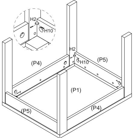
Attach 4 x Bracket (H2) to Rails (P5x2) and Legs and secure with 8 x Screws (H10) by tightening with a Phillips Head Screwdriver.
