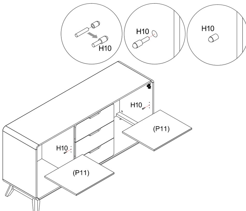
Insert 8 x Shelf Pins (H10) into desired holes in panels.
