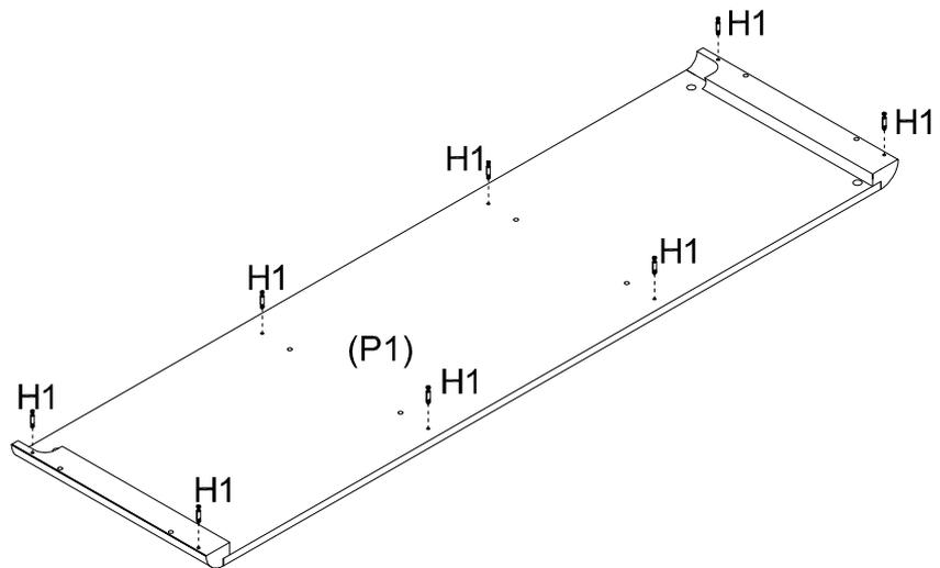
Screw 8 x Cam Bolts (H1) into Top Panel (P1) as shown.
