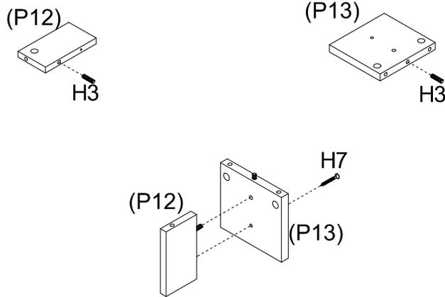
Insert 2 x Wood Dowels (H3) into Small Middle Leg (P12) and Big Middle Leg (P13).
