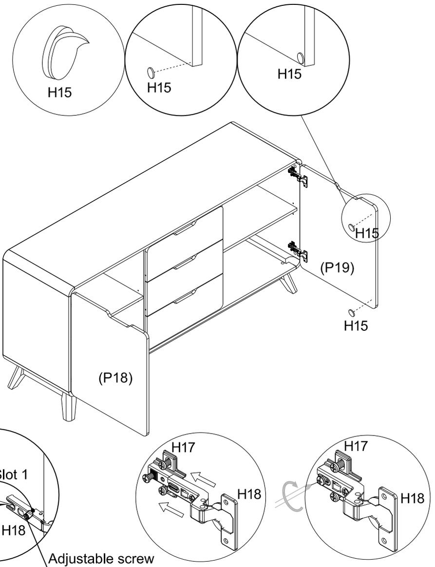
Attach doors onto cabinet as shown. Slide Hinge (H18) onto Hinge Base (H17), until each adjustable screw is in slot 1 and the lock screw is in the slot 2, then tighten lock screw. Attach 4 x Pads (H15) onto Doors (P15) and (P16).
