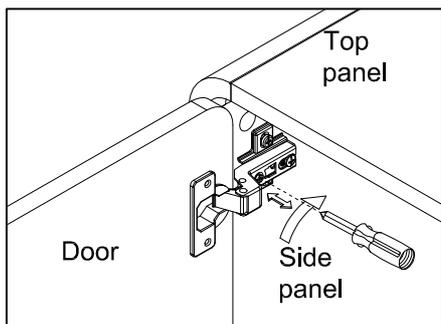
Loosen or tighten the screw indicated a little to adjust the gap between the door panels, adjust the hinge to right position (see step 3a & 3b).
