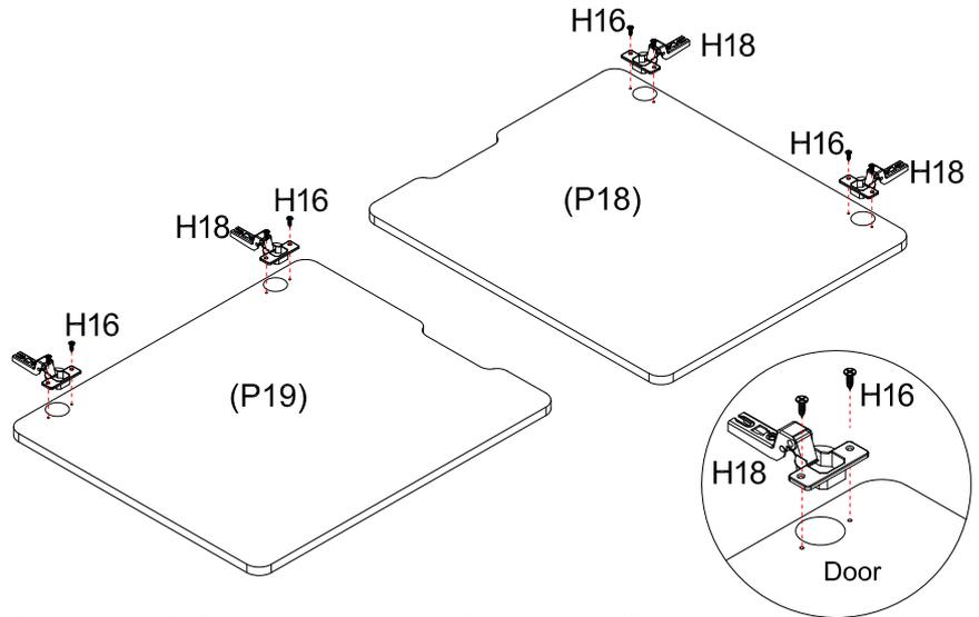
Insert 4 x Hinges (H18) into Doors (P18) and (P19). Attach with 8 x Screws (H16).
