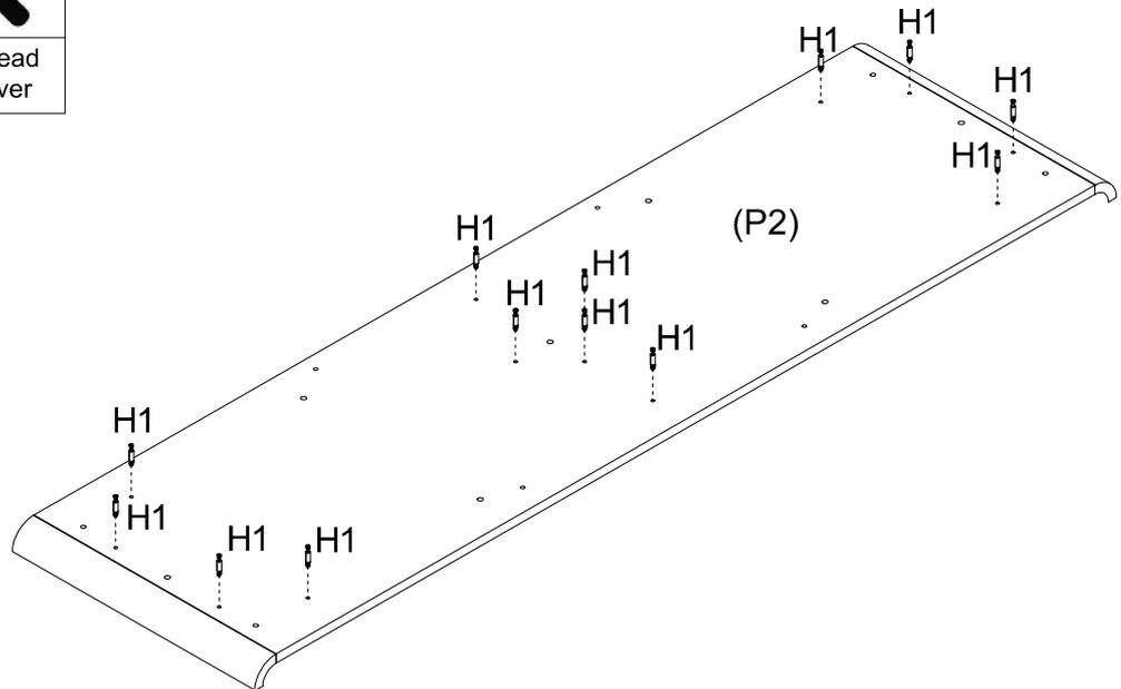
Screw 13 x Cam Bolts (H1) into Bottom Panel (P2) as shown.
