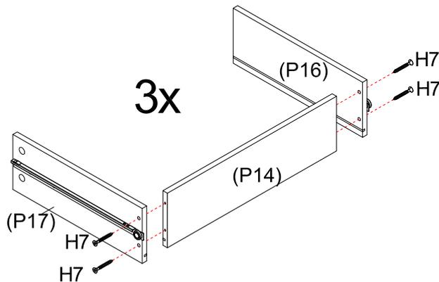
Attach each Drawer Side Panels (P16) and (P17) to each Drawer Back (P14) with 4 x Screws (H7). Repeat two times for all drawer panels.
