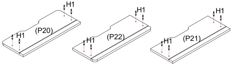
Screw each 4 x Cam Bolts (H1) into Drawer Fronts (P20) (P21) (P22) using a Phillips head screwdriver.
