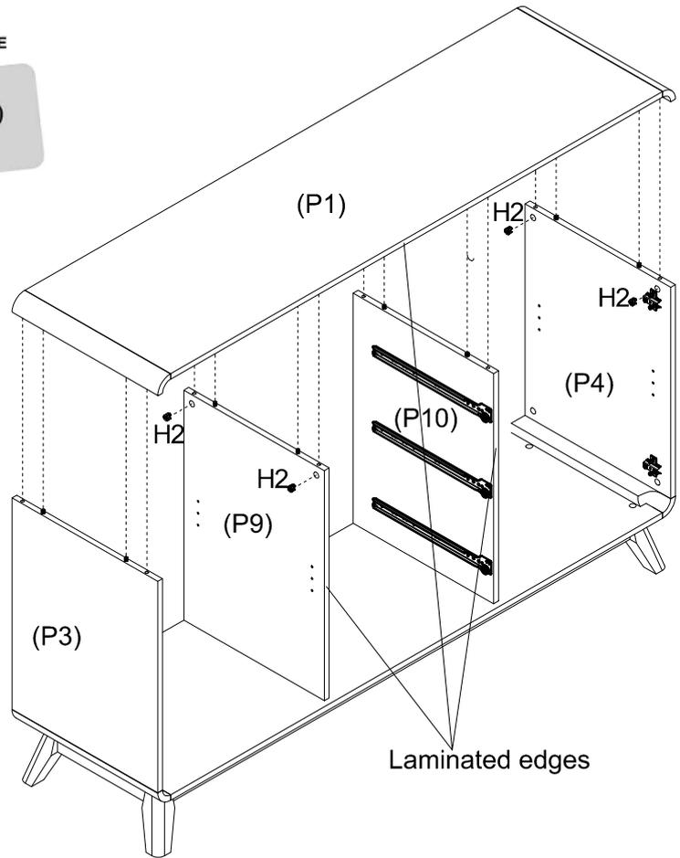
Attach Top Panel (P1) to Side Panels (P3) & (P4) and Divider Panels (P9) & (P10). Make sure the laminated edges of Top Panel (P1), Divider Panels (P9) and (P10) face all the same direction. Insert 8 x Big Cam Nuts (H2) into Side Panels (P3), (P4) and Divider Panels (P9), (P10) and turn clockwise to lock.
