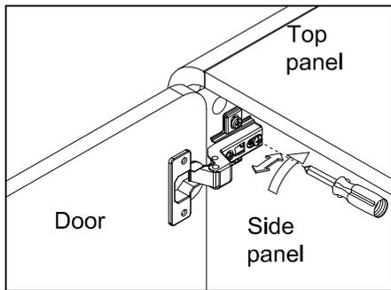
Loosen the screw indicated a little, adjust the hinge to right position (see step 2a & 2b), then tighten the screw.
