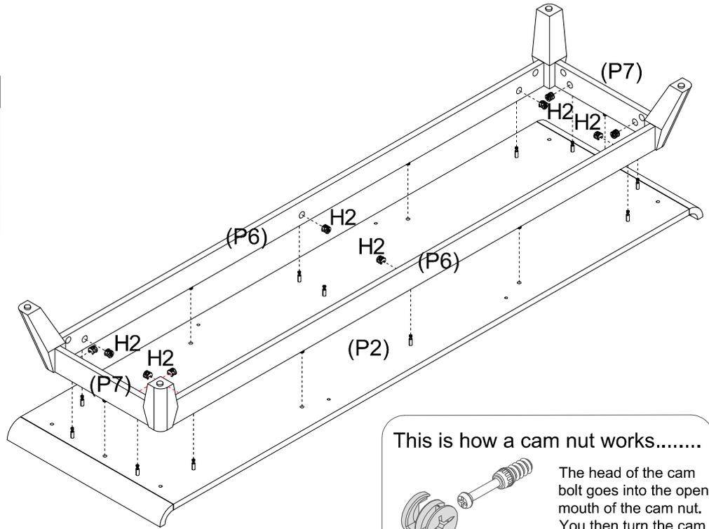
This is how a cam nut works.....
