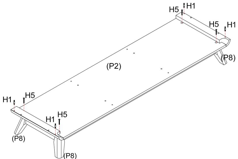
Screw 4 x Cam Bolts (H1) into Bottom Panel (P2) as shown.
