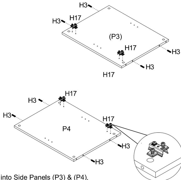
Insert 8 x Wood Dowels (H3) into Side Panels (P3) & (P4). Attach 4 x Hinge Bases (H17) to Side Panels, tighten all screws with a phillips head screwdriver.
