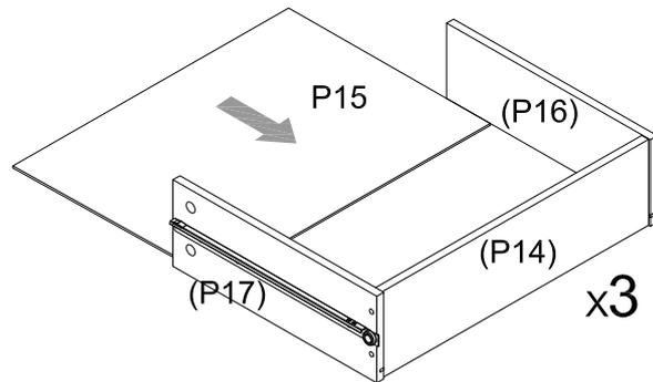
Slide each Drawer Base (P15) into the groove in the Drawer Panels (P17), (P16) and (P14). Repeat two times for all Drawer Bases (P15).
