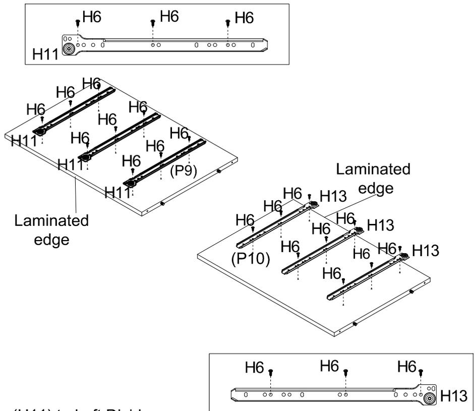
Attach 3 x Left Runner Tracks (H11) to Left Divider Panel (P9) with 9 x Screws (H6).
