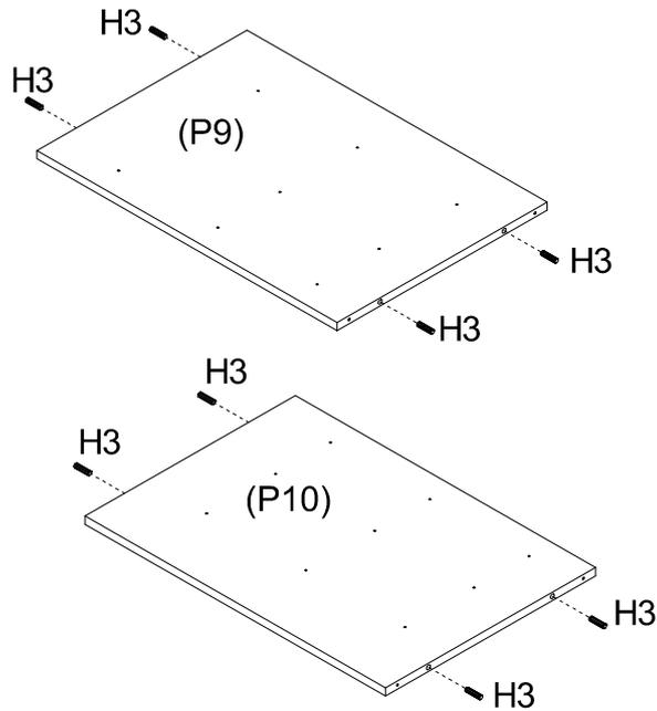
Insert 8 x Wood Dowels (H3) into Divider Panels (P9) and (P10).
