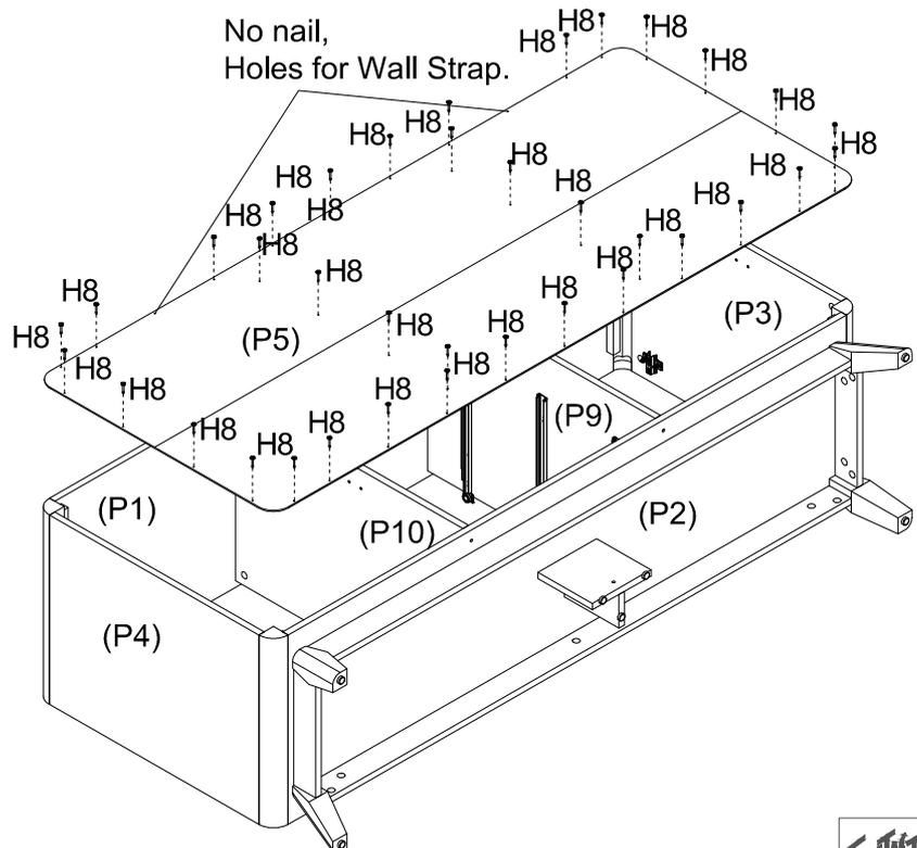
Attach Back Panel (P5) to Panels (P1) (P2) (P3) (P4) (P9) and (P10) with 36 x Nails (H8).
