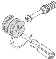
The head of the cam bolt goes into the open mouth of the cam nut. You then turn the cam nut so it tightens over the bolt.
