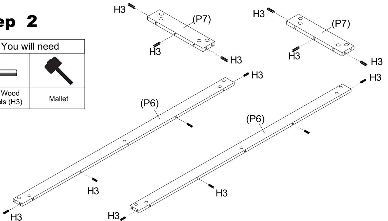
Insert each 3 x Wood Dowels (H3) into Short Rail (P7) and each 4 x Wood Dowels (H3) into Long Rail (P6).
