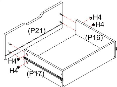
Attach Drawer Front (P20) to Drawer Sides (P17) & (P16). Insert 4 x Small Cam Nuts (H4) into Drawer Sides (P17) & (P16). Rotate the cam nuts so the arrows point towards the incoming cam bolt and turn clockwise to lock. Repeat for other Drawer Fronts (P21) & (P22).
