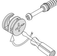
The head of the cam bolt goes into the open mouth of the cam nut. You then turn the cam nut so it tightens over the bolt.
