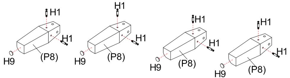
Screw each 2 x Cam Bolts (H1) into Leg (P8) using a phillips head screwdriver.
