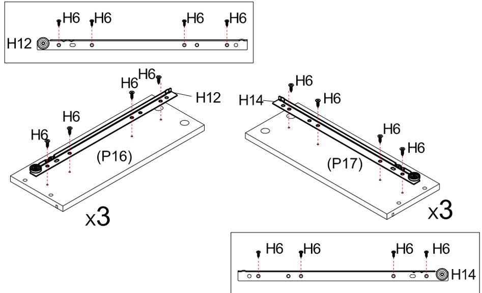
Attach each one Left Runner (H12) to Left Drawer Sides (P16) with 4 x Screws (H6). Repeat two times for all Left Drawer Sides (P16).
