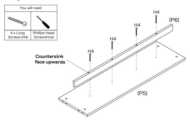
Attach Rail (P6) to Shelf Panel (P5) with 4 x Long Screws (H4) by tightening with the Phillips Head Screwdriver.
