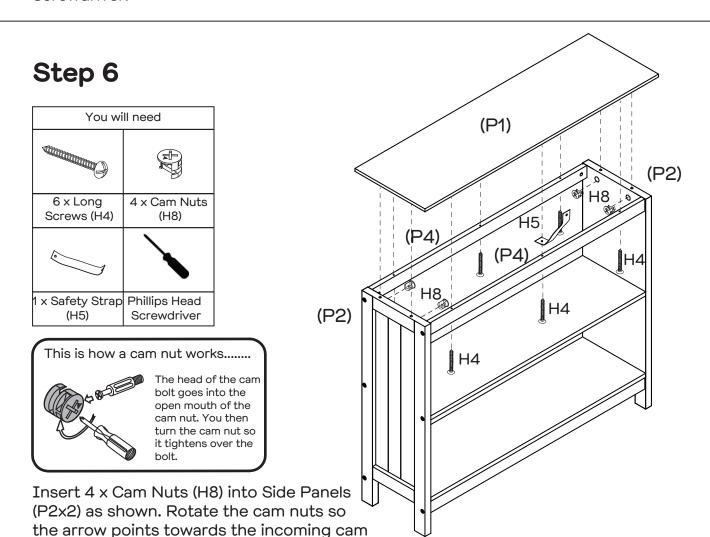
bolts. Attach 1 x Safety Strap (H5) between Top Panel (P1) and Rail (P4) as shown. Attach Rails (P4x2) and Side Panels (P2x2) to Top Panel (P1) with 6 x Long Screws (H4) by tightening with the Phillips Head Screwdriver.
