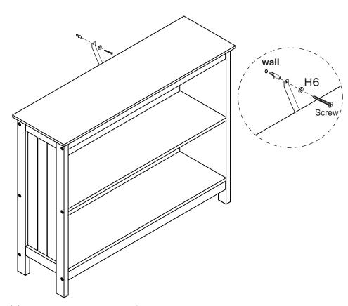
Move the hall table to the final position, and attach the safety strap to the wall securely. Make sure it is firmly attached and snug fit.
