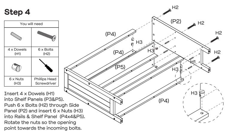
Attach Rails & Shelf Panel (P4x4&P5) to Side Panel (P2) by tightening all nuts with the Phillips Head Screwdriver.
