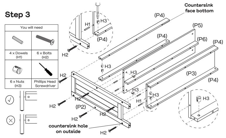
Insert 4 x Dowels (H1) into Shelf Panels (P3&P5). Push 6 x Bolts (H2) through Side Panel (P2) and insert 6 x Nuts (H3) into Rails & Shelf Panel (P4x4&P5). Rotate the nuts so the opening point towards the incoming bolts. Attach Rails & Shelf Panel (P4x4&P5) to Side Panel (P2) by tightening all nuts with the Phillips Head Screwdriver.
