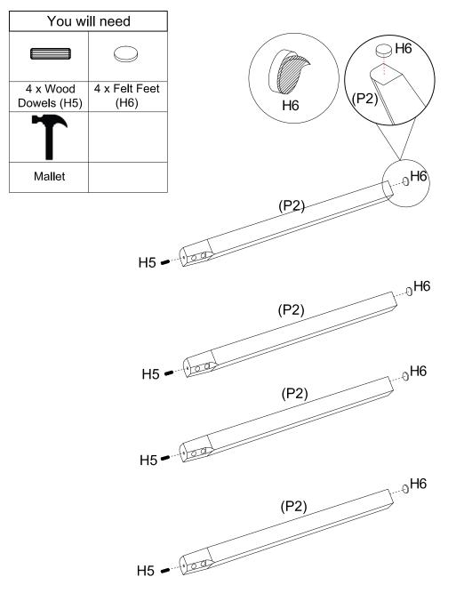
Insert each Wood Dowel (H5) into leg (P2). Attach each Felt Feet (H6) onto Leg (P2).
