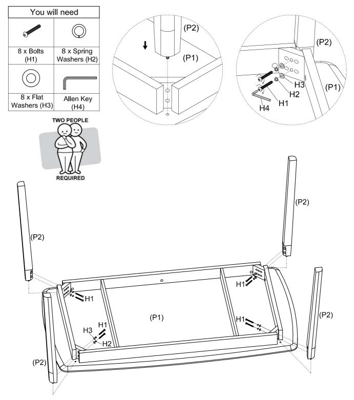
Attach Leg (P2) onto Top (P1) using 2 x Bolts (H1), 2 x Flat Washers (H3) and 2 x Spring Washers (H2). Tighten the bolt with Allen Key (H4). Repeat three times for all Legs (P2).
